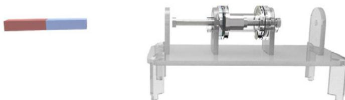
Rotate the bar magnet by moving the mouse across the screen from left to right. As the poles of the bar magnet alternate, the magnet in the motor on the right moves back and forth as it is alternately attracted and repelled by the changing polarity of the bar magnet.
