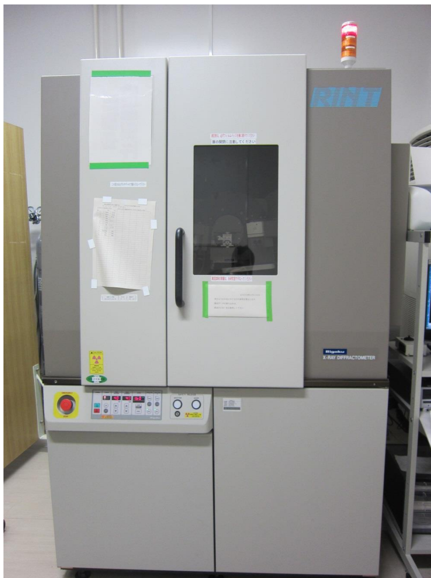
Fig. 2. 2. Rigaku X-ray diffractometer at Center for Nanodevice Fabrication and Analysis, Shizuoka University
