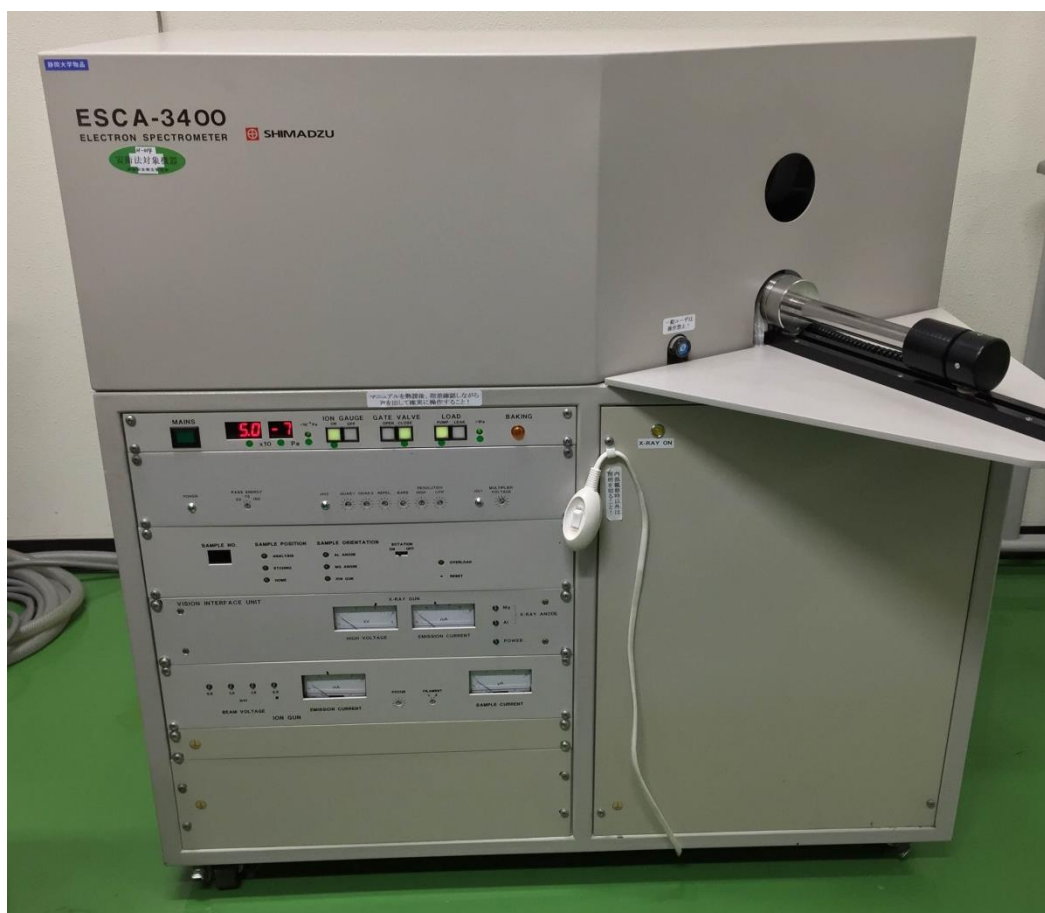
Fig. 2. 5. Shimadzu ESCA 3100 spectrophotometer X-ray photoelectron spectroscopy
