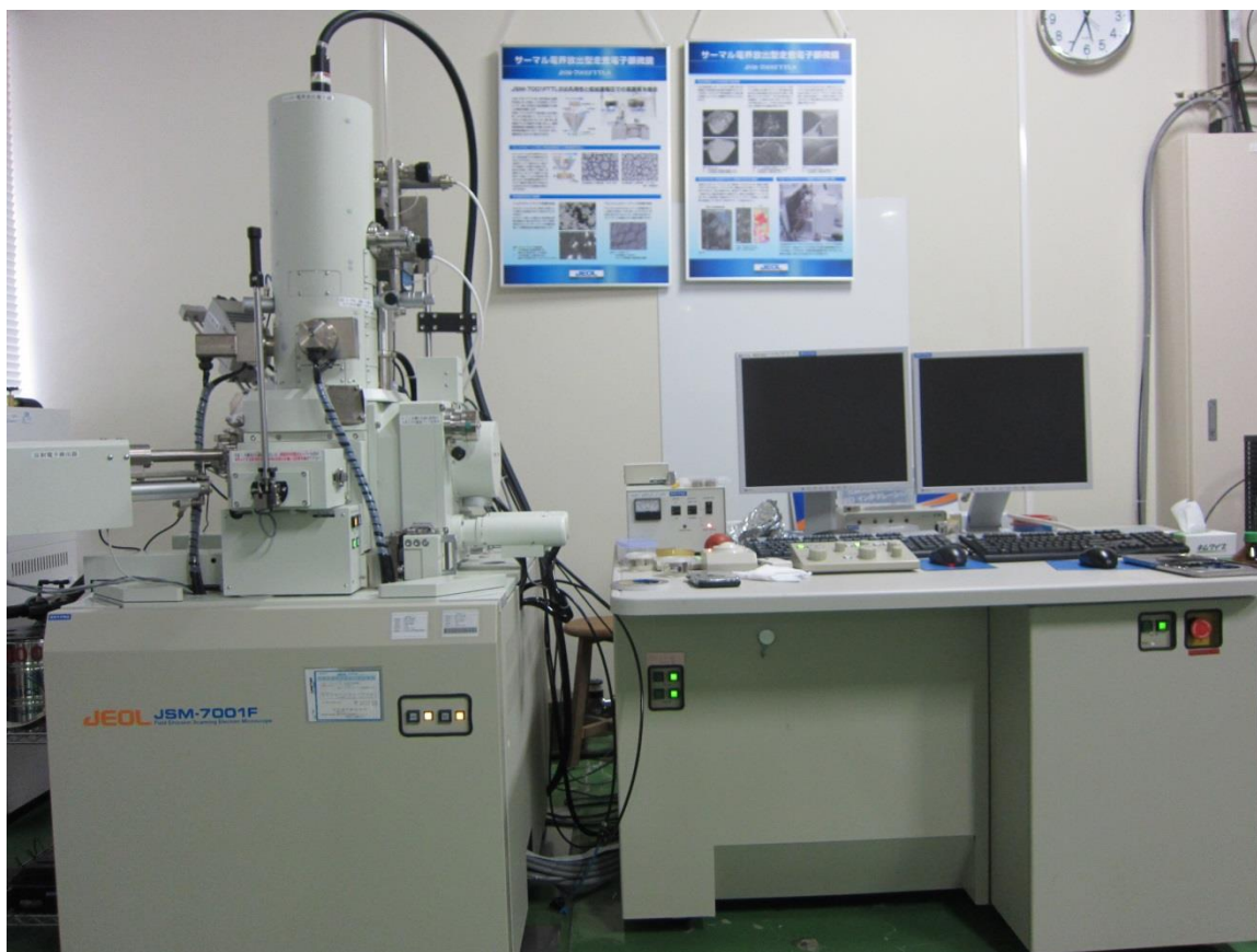
Fig. 2. 3. JEOL – JSM 7001F field emission scanning electron microscope at Center for Instrumental Analysis, Shizuoka University
