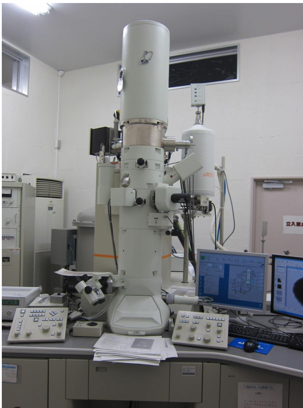
Fig. 2. 4. JEOL JEM 2100F transmission electron microscope at Center for Nanodevice Fabrication and Analysis, Shizuoka University.
