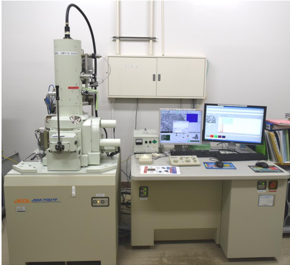
Figure 2.5 JEOL - JSM 7001F field emission scanning electron microscope at Center for Nano device Fabrication and Analysis, Shizuoka University
