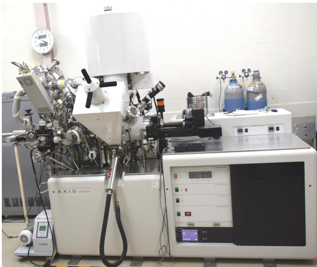
Figure 2.4 XPS (AXIS ULTRA DLD) X-ray photoelectron spectroscopy at Center for Nano device Fabrication and Analysis, Shizuoka University
