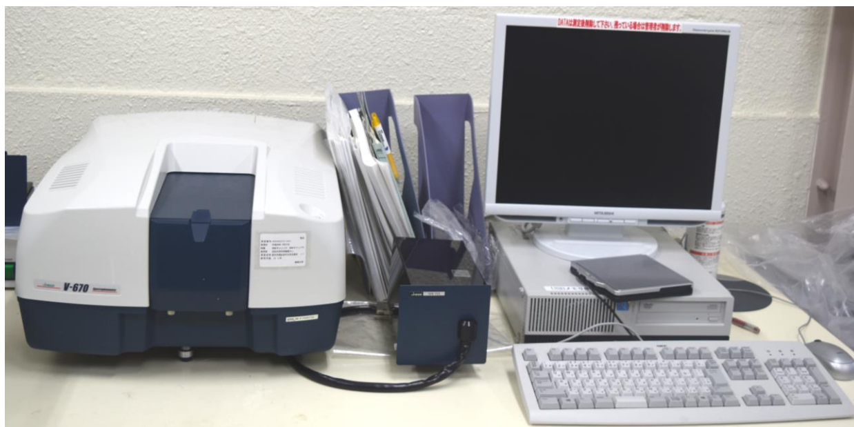
Figure 2.3 Jasco UV-Vis (V-670) UV visible absorptions spectrophotometer at Center for Nano device Fabrication and Analysis, Shizuoka University
