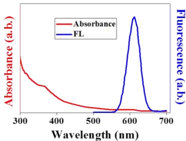
**Fig. S2.** UV/Vis spectrum (red spectrum) and FL spectrum (blue spectrum) of CdSeInS QD.
