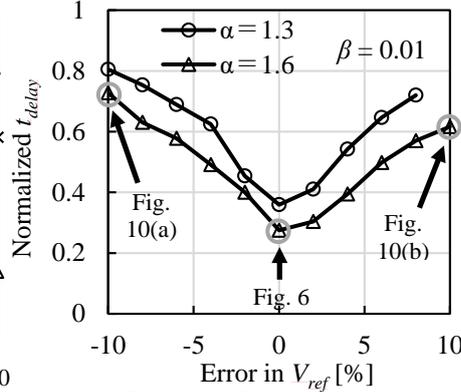
Fig. 9 (a). Impact of errors in  $V_{ref}$  on  $t_{delay}$  ( $\beta = 0.01$ )
