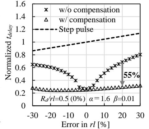
Fig. 14. Impact of errors in RC product on  $t_{delay}$
