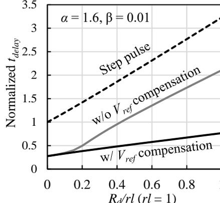
Fig. 13. Influence of  $R_d$  on delay time
