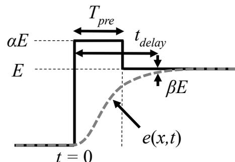
Fig. 2. Pre-emphasis pulse and the definition of the design parameters
