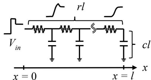
Fig. 1. Equivalent circuit of RC delay line (WL or CL)
