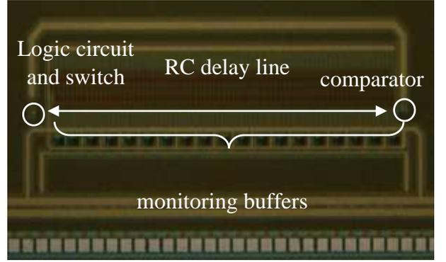
Fig. 5. Chip micrograph
