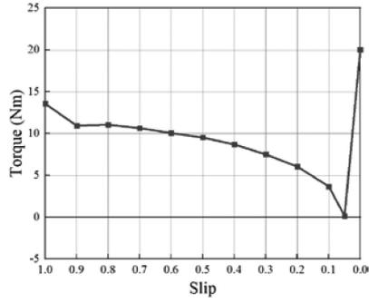
Fig. 5. Slip-vs.-torque characteristics under  $100 V_{\text{rms}}$ . (FE-analysis results).
