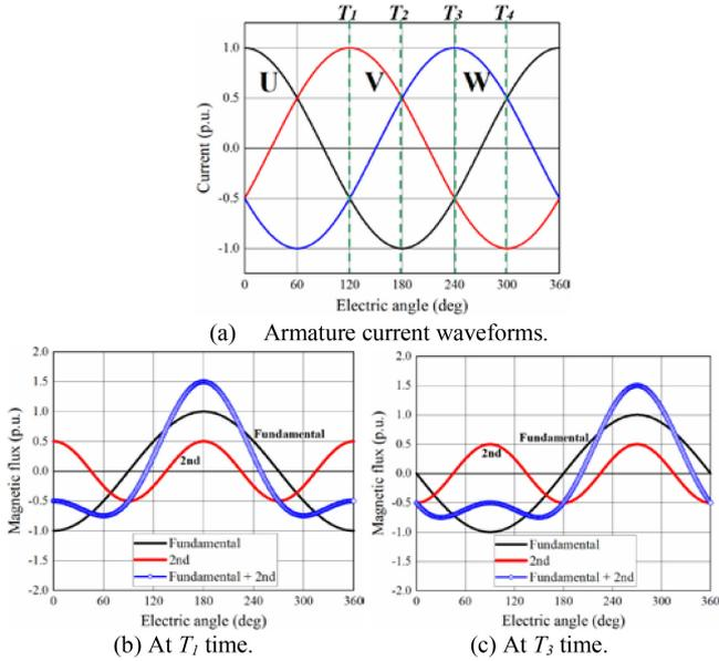
Fig. 3. Armature current waveforms and special magnetic force waveforms.
