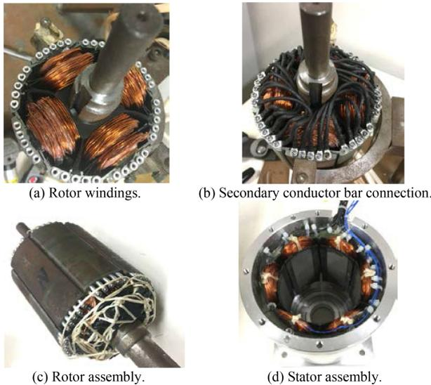
Fig. 8. Actual prototype machine.
