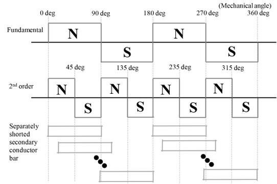
Fig. 4. Separately shorted secondary conductor bar with pole-pitch.
