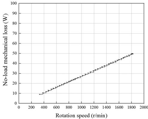
Fig. 12. Mechanical loss at no-load.
