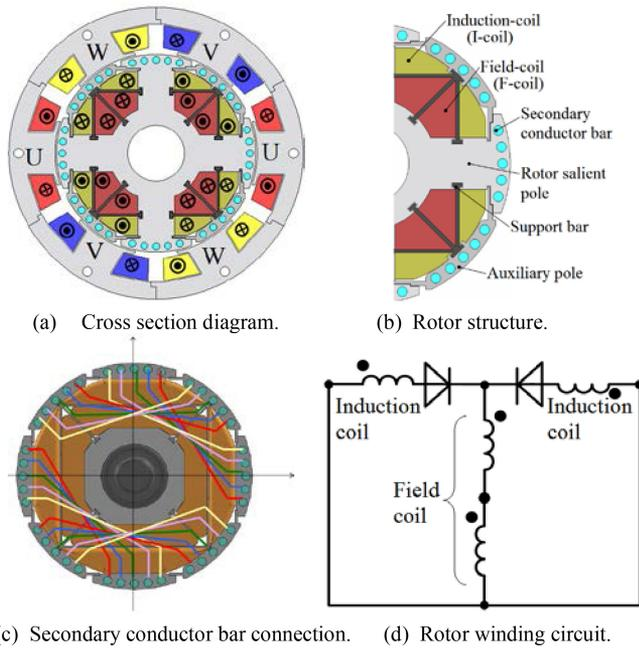
Fig. 1. Proposed novel line-start machine.
