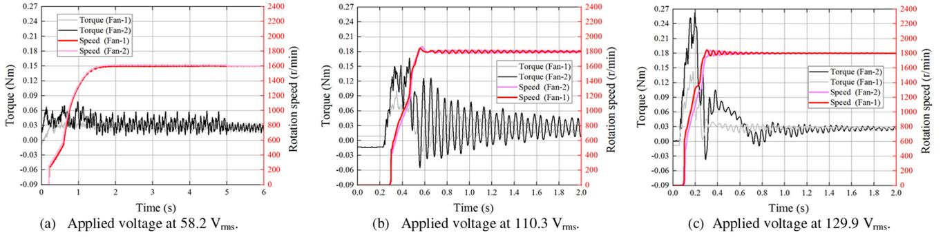
Fig. 10. Line start characteristics with respect to applied voltage under fan loads.
