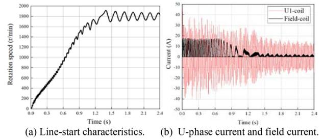
Fig. 6. U-phase and field current at applied voltage  $70.7 V_{\text{rms}}$  under no-load line start. (FE-analysis results).
