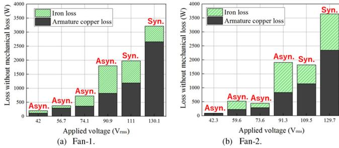
Fig. 11. Measured loss with respect to applied voltage under fan loads.
