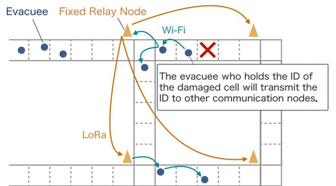
Fig. 3 Cellular automaton communication model ( $R_{wlan} = 2, R_{loran} = 20$ ).
