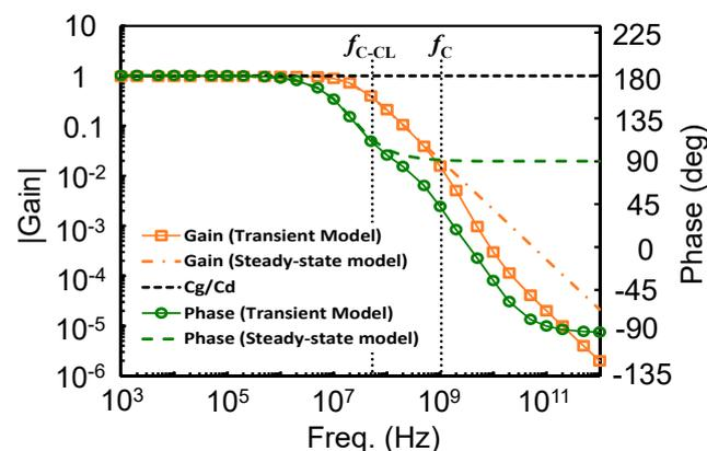
Figure 11. The frequency response of the SET inverting amplifier with a load capacitor  $C_L = 30$  aF ( $10 C_\Sigma$ ) operating at a drain current  $I_d = 26.4$  pA, gate voltage  $V_{gs} = 53.4$  mV [0.33] (center of the descending side of the CD) and  $T = 15.5$  K [0.05].
