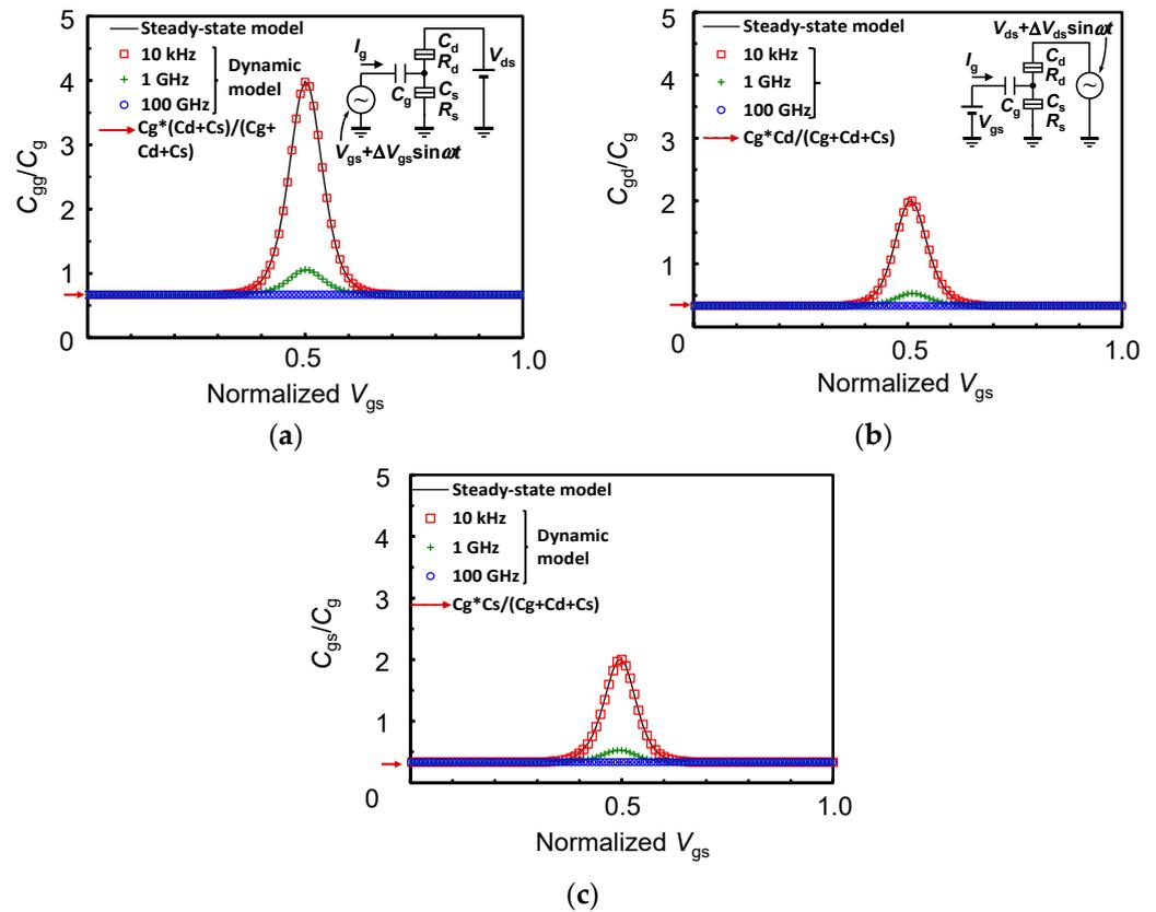
**Figure 3.** (a) SET input capacitance  $C_{gg}$  (b) drain-to-gate capacitance  $C_{gd}$  and (c) source-to-gate capacitance  $C_{gs}$  as a function of gate voltage  $V_{gs}$  for a low drain voltage  $V_{ds} = 0.534$  mV [0.01] at  $T = 15.5$  K [0.05].
