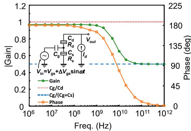
**Figure 8.** Frequency response of the SET inverting amplifier operating at a drain current  $I_d = 26.4$  pA, gate voltage  $V_{gs} = 53.4$  mV [0.33] (center of the descending side of the CD) and  $T = 15.5$  K [0.05].
