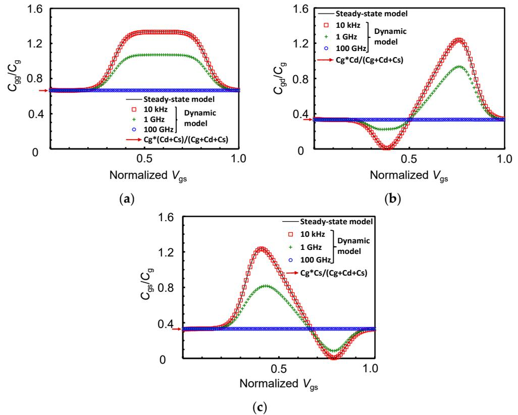
**Figure 4.** (a) SET input capacitance  $C_{gg}$  (b) drain-to-gate capacitance  $C_{gd}$  and (c) source-to-gate capacitance  $C_{gs}$  as a function of gate voltage  $V_{gs}$  for a high drain voltage  $V_{ds} = 26.7$  mV [0.5] at  $T = 15.5$  K [0.05].
