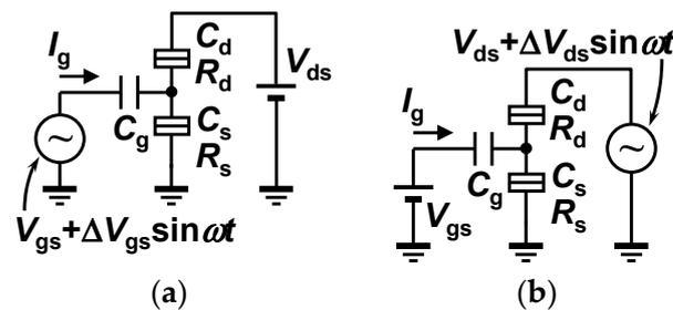
Figure 2. Circuit diagrams for the measurement of (a)  $C_{gg}$  and (b)  $C_{gd}$ .
