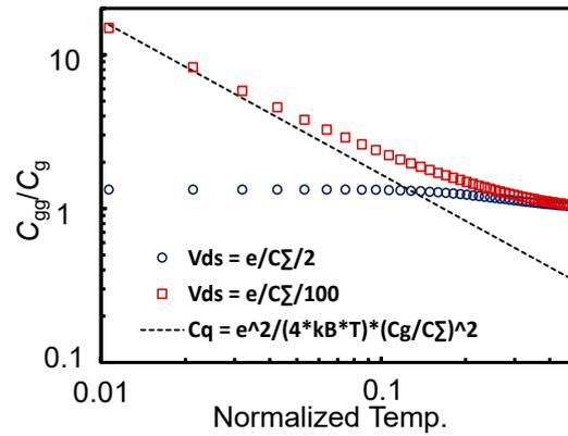
**Figure 6.** SET input capacitance  $C_{gg}$  as a function of temperature at drain voltages  $V_{ds} = 0.534$  mV [0.01] and 26.7 mV [0.5], and gate voltages  $V_{gs} = 80.1$  mV [0.5] and 93.5 mV [0.6], respectively.
