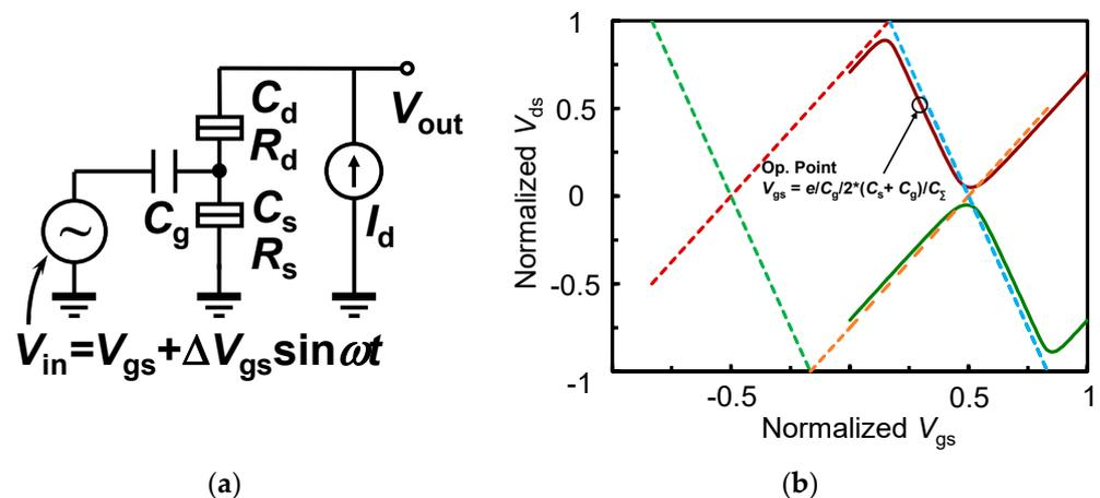
**Figure 7.** (a) A circuit diagram of the SET-based inverting amplifier with constant-current load, and (b) Coulomb diamond (CD) plot with  $V_{ds}-V_{gs}$  curves for  $I_d = \pm 26.7$  pA at  $T = 15.5$  K [0.05]. The operation point of the amplifier is set at the center of the descending side.
