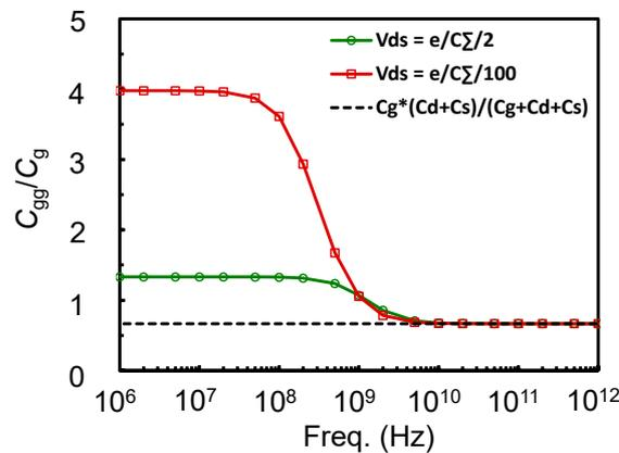
**Figure 5.** SET input capacitance  $C_{gg}$  as a function of frequency at drain voltages  $V_{ds} = 0.534$  mV [0.01] and  $26.7$  mV [0.5], gate voltages  $V_{gs} = 80.1$  mV [0.5] and  $93.5$  mV [0.6] and  $T = 15.5$  K [0.05].
