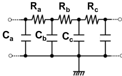
Fig. 3.4: Distributed CR filter model to calculate the frequency response of the parasitic component (lead). Note that each section *a*, *b* or *c* is further divided into 10 subsections to properly simulate the distributed circuit characteristics [8].
