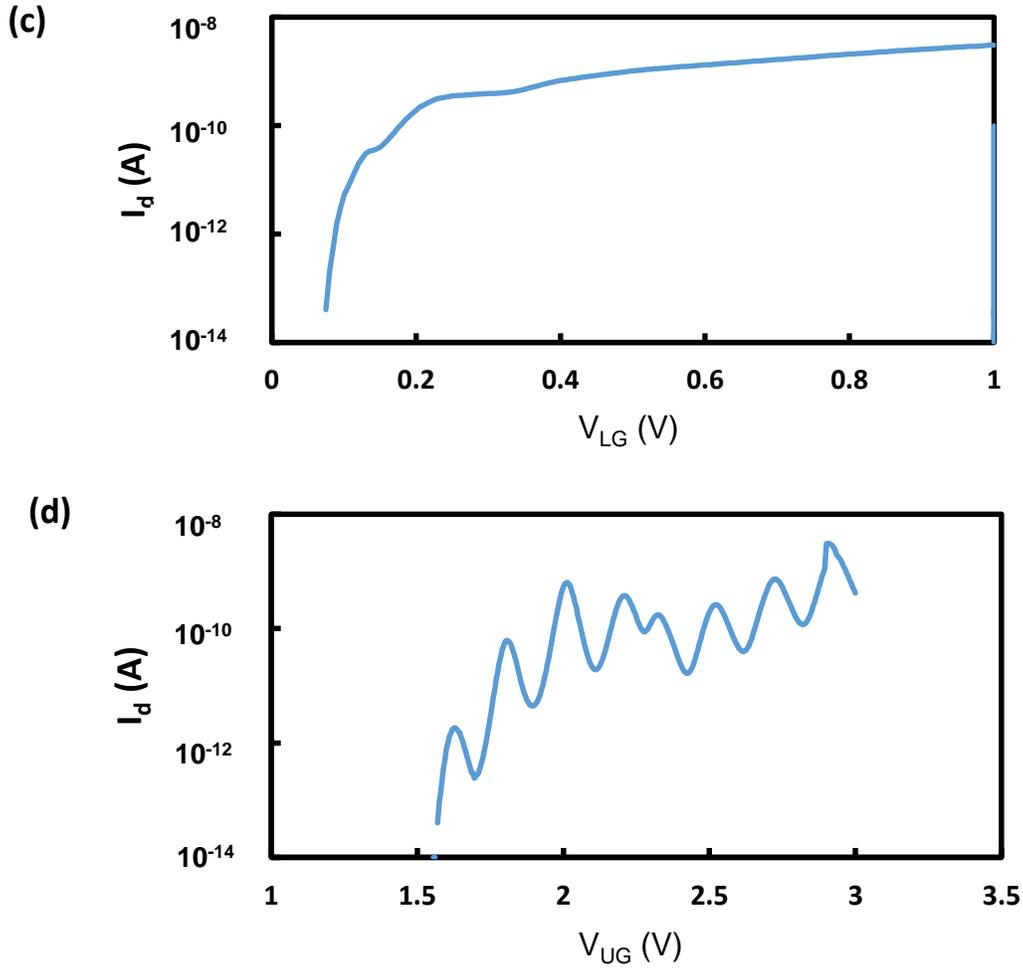
Fig. 3.3:  $I_d$ - $V_g$  Characteristics of device type 1 (a) with lower and upper gate, L50 nm W50 nm (b) with only upper gate, L50 nm W 44 nm; device type 2 (c) with lower and upper gate L50 nm W 50 nm (d) with only upper gate: L50 nm W 44 nm
