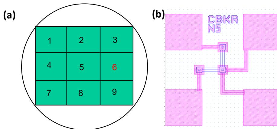
Fig. 3.24: (a) Si wafer layout of SET devices with multiple island channel
