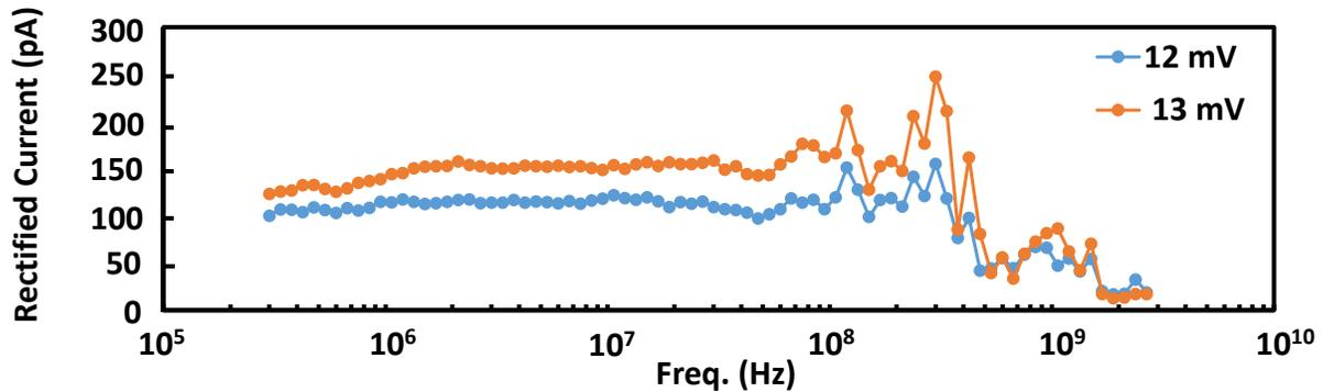
Fig. 3.16: Frequency response of the rectified current
