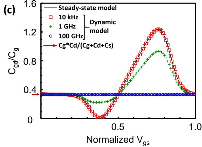
Fig. 2.13: (a) SET input capacitance  $C_{gg}$  (b) drain-to-gate capacitance  $C_{gd}$  and (c) source-to-gate capacitance  $C_{gs}$  as a function of gate voltage  $V_{gs}$  at drain voltage  $V_{ds} = 26.7$  mV [0.5] and temperature  $T = 15.5$  K [0.05]
