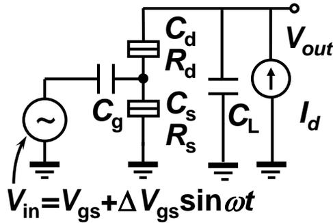
Fig. 2.21: Circuit diagram of the SET-based inverting amplifier with constant-current load and load capacitance  $C_L$
