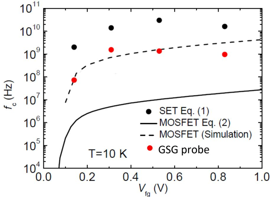
Fig. 3.5: Cutoff frequency of SET and parasitic MOSFETs [6], [7], [8]
