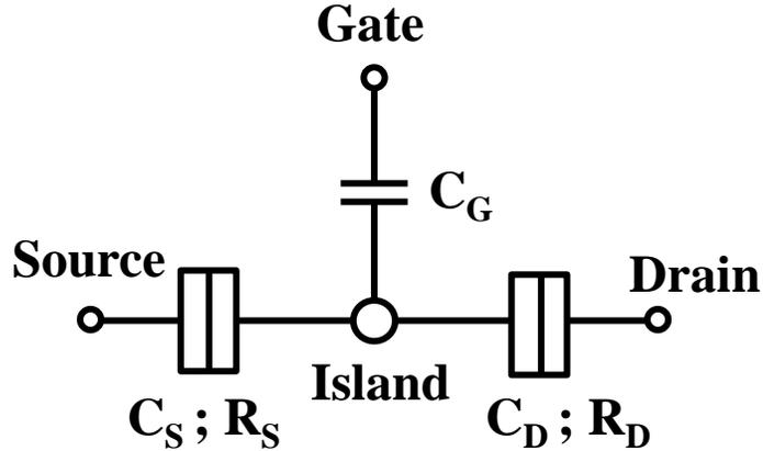
Fig. 1: Schematic diagram of basic SET
