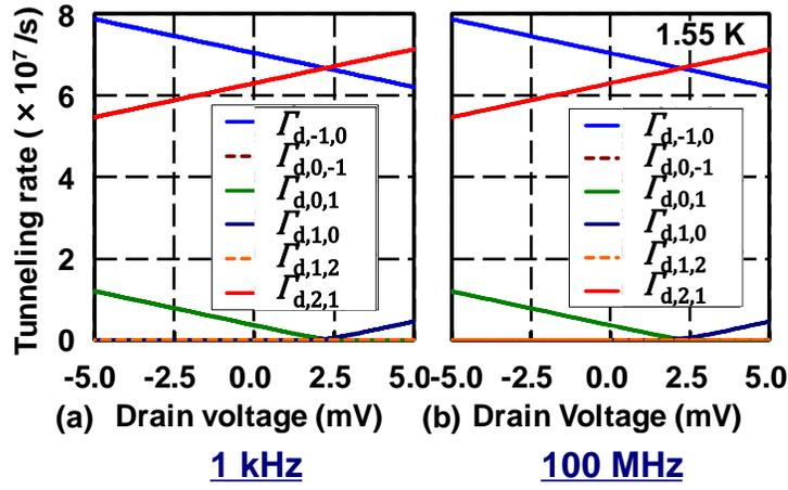
Fig. 2.7: Tunneling rate vs. drain voltage at (a) low frequency (1 kHz), and (b) high frequency (100 MHz).
