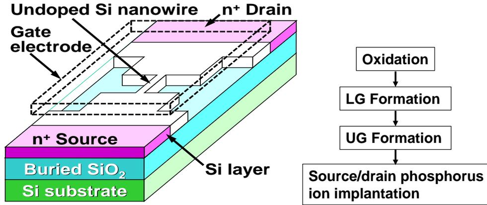
Fig. 3.1: Silicon SET fabricated by PADOX method along with fabrication steps
