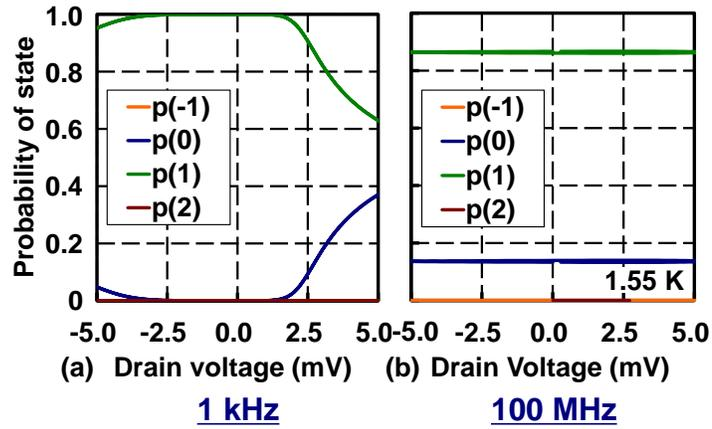
Fig. 2.5: Probability of state vs drain voltage at (a) low frequency (1 kHz) and (b) high frequency (100 MHz)
