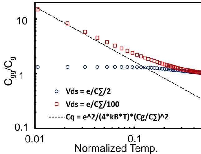
Fig. 2.16: Gate input capacitance  $C_{gg}$  as a function of temperature at drain voltage  $V_{ds} = 0.534$  mV [0.01] and 26.7 mV [0.5], gate voltage  $V_{gs} = 80.1$  mV [0.5] and 93.5 mV [0.6] and temperature  $T = 15.5$  K [0.05]
