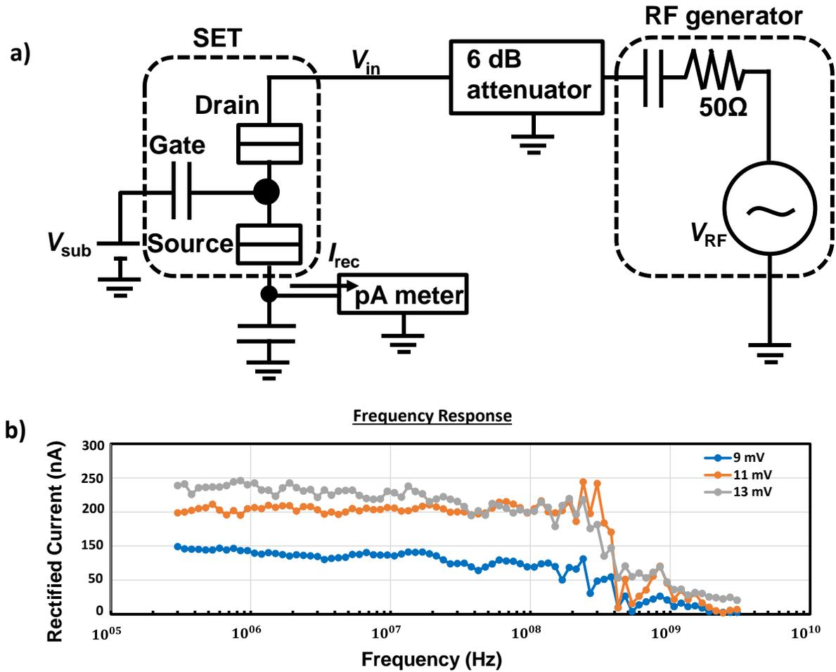
Fig. 3.9: (a) Modified high-frequency measurement setup for rectifying current (b) frequency response of SET having  $L = 52$  nm and  $W = 92$  nm and RF signal amplitude 9, 11 and 13 mV
