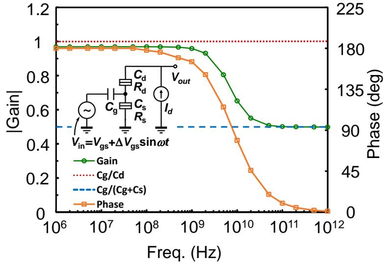
Fig. 2.18: Frequency response of SET inverting amplifier operating at drain current  $I_d = 26.4$  pA, gate voltage  $V_{gs} = 53.4$  mV (center of the descending side of the Coulomb diamond) and temperature  $T = 15.5$  K [0.05].in SET.
