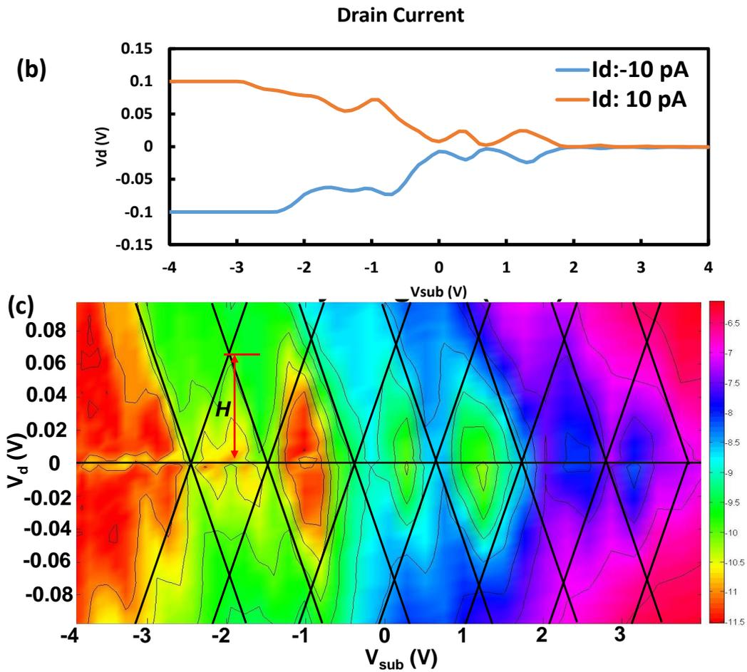
Fig. 3.14: (a)  $I_d$ - $V_{sub}$  (b)  $V_d$ - $V_{sub}$  and (c) Stability diagram of SET (L:52 ; W: 92 nm) at  $T = 20$  K
