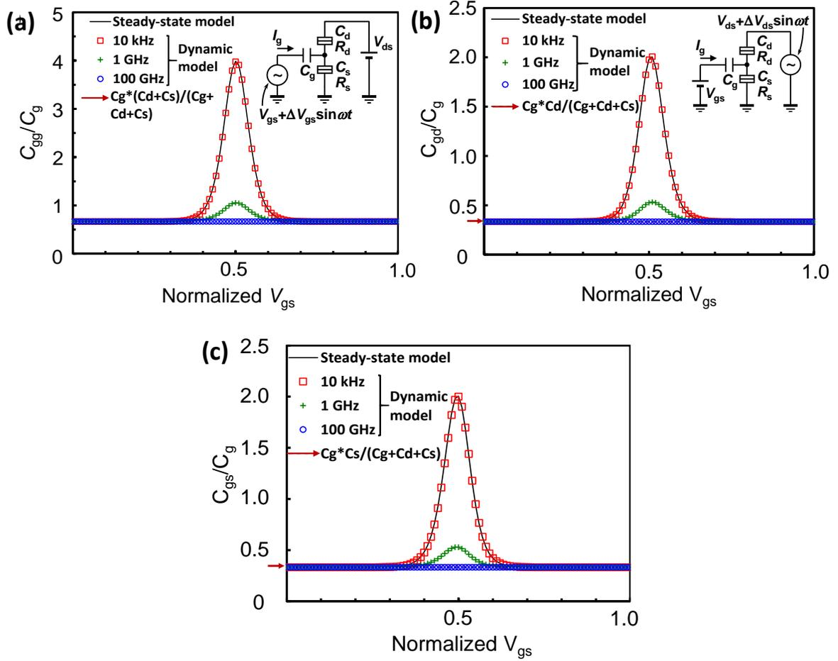
Fig. 2.12: (a) SET input capacitance  $C_{gg}$  (b) drain-to-gate capacitance  $C_{gd}$  and (c) source-to-gate capacitance  $C_{gs}$  as a function of gate voltage  $V_{gs}$  at drain voltage  $V_{ds} = 0.534$  mV [0.01] and temperature  $T = 15.5$  K [0.05]
