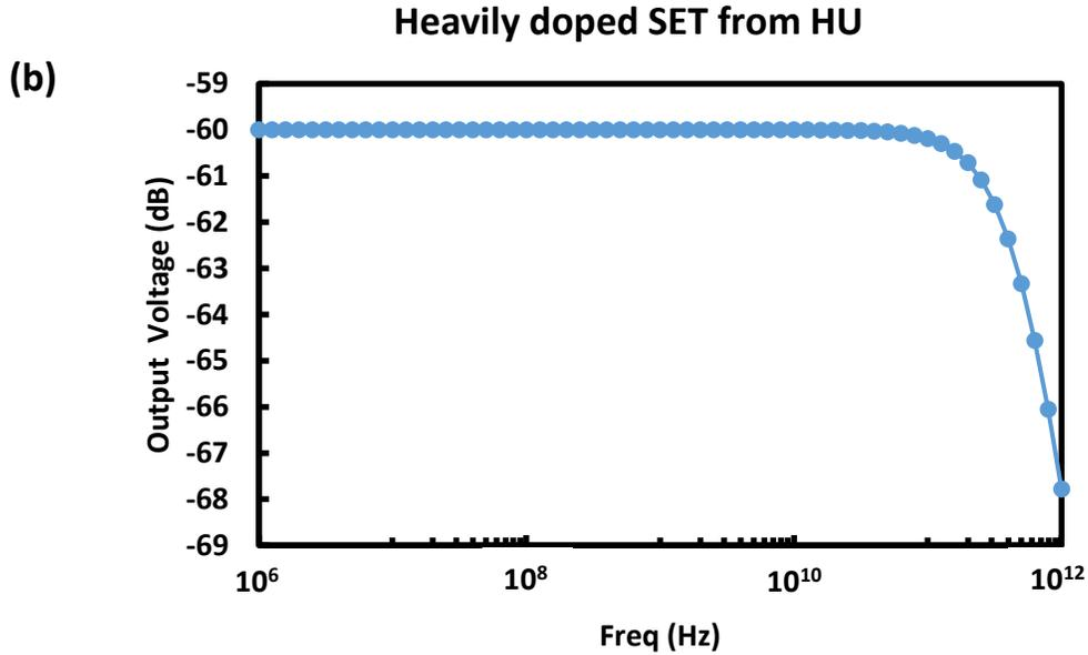
Fig. 3.7: Cutoff frequency of distributed CR filter of (a) Heavily doped SET from SU (b) Heavily doped SET from HU
