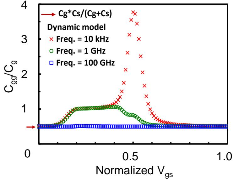
Fig. 2.19: SET input capacitance  $C_{gg}$  as a function of gate voltage  $V_{gs}$  at drain current  $I_d = 26.7$  pA and temperature  $T = 15.5$  K [0.05]
