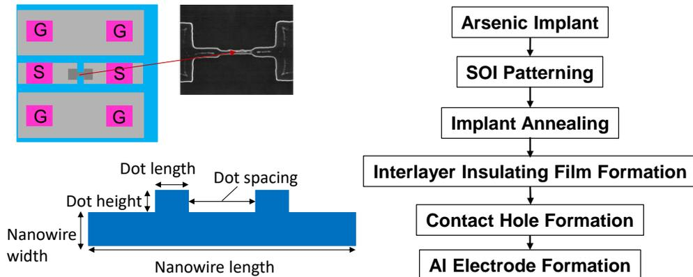
Fig. 3.18: Schematic of Si SET with multiple islands along with fabrication step
