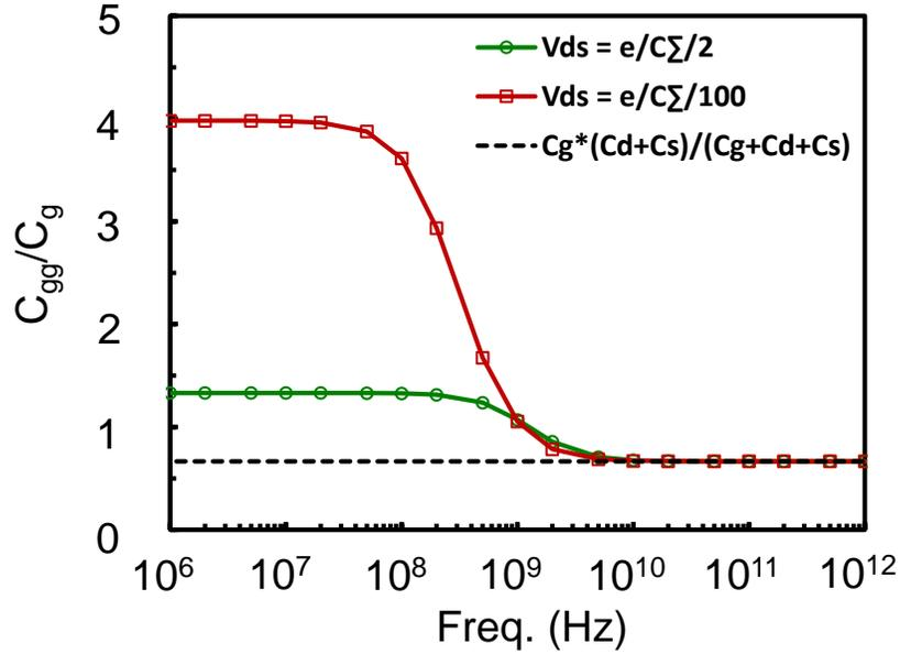
Fig. 2.15: Gate input capacitance  $C_{gg}$  as a function of frequency at drain voltage  $V_{ds} = 0.534$  mV [0.01] and 26.7 mV [0.5], gate voltage  $V_{gs} = 80.1$  mV [0.5] and 93.5 mV [0.6] and temperature  $T = 15.5$  K [0.05].
