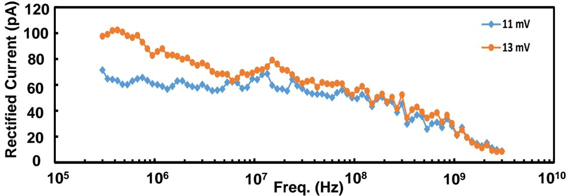
Fig. 3.23: Frequency response of the rectified current
