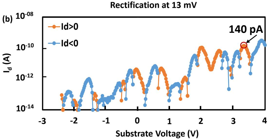
Fig. 3.15: Rectified current  $I_d$  as a function of substrate voltage  $V_{sub}$  at AC signal 1 MHz and amplitude (a) 12 mV and (b) 13 mV
