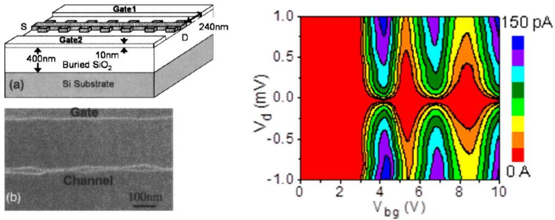
Fig. 3.17: SET with multiple channel island structure [16], [17].
