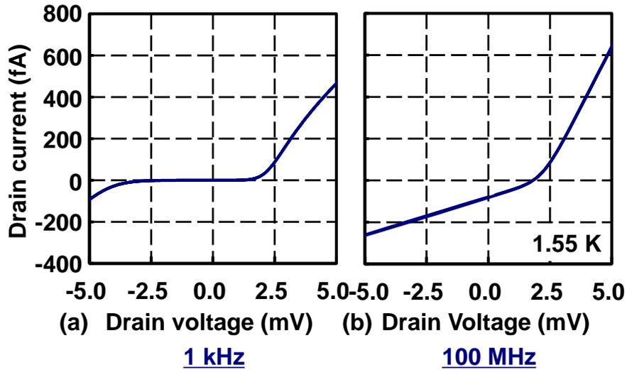
Fig. 2.8: Drain current vs. drain voltage at (a) low frequency (1 kHz), and (b) high frequency (100 MHz).
