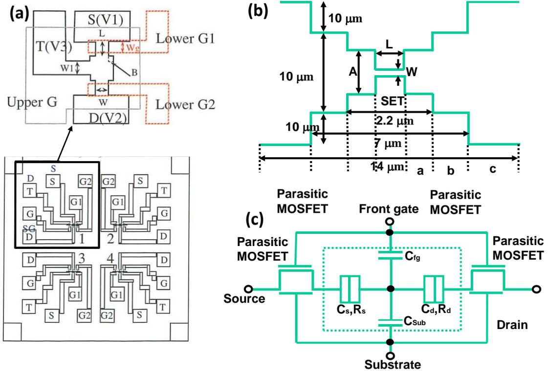
Fig. 3.2: (a) Layout of silicon SET fabricated by PADOX method
