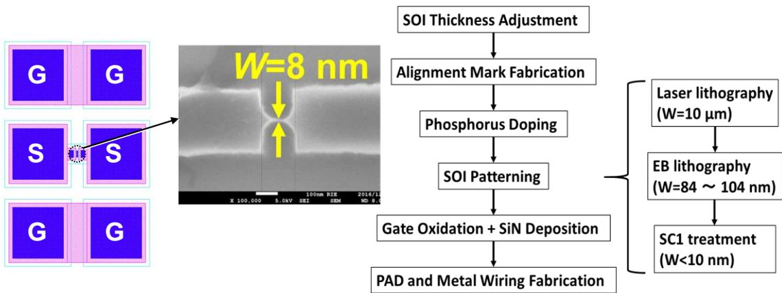
Fig. 3.12: Schematic of heavily doped silicon nanowire-based SET along with fabrication step
