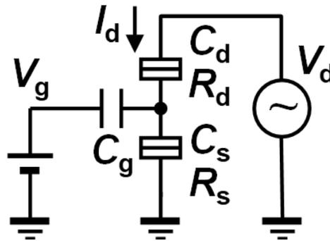
Fig. 2.2: Schematic circuit diagram to operated SET as a rectifier
