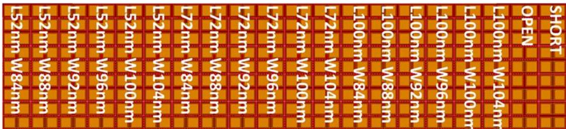
Fig. 3.13: Heavily doped silicon nanowire-based SET layout with different dimensions
