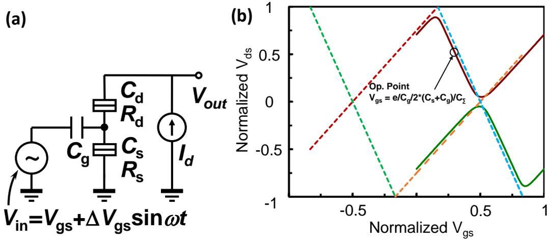
Fig. 2.17: (a) Circuit representation of SET as a voltage amplifier and (b) Corresponding operation point in  $V_{ds}$ - $V_{gs}$  graph at drain voltage  $I_d = \pm 26.7$  pA.
