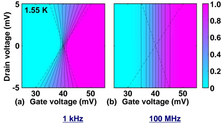
Fig. 2.6: Contour plots of the number of electrons in the Coulomb island at (a) low frequency (1 kHz), and (b) high frequency (100 MHz). Dashed lines represent the boundary of the Coulomb diamond set by the capacitance parameters  $C_g$ ,  $C_d$  and  $C_s$ .
