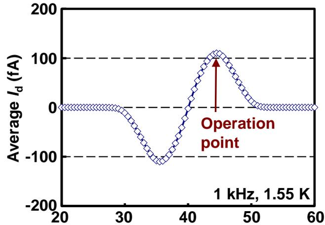
Fig. 2.3: Rectifying current vs. gate voltage  $V_g$ .  $C_g=C_d=C_s=2.0$  aF,  $R_d=R_s=2.5$  G $\Omega$ ,  $V_d=\pm 5.34$  mV<sub>p-p</sub> [0.2],  $T=1.55$  K [0.01].
