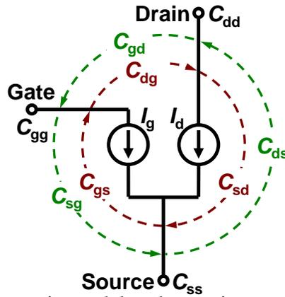
Fig. 2.10: Schematic model and capacitance components in SET
