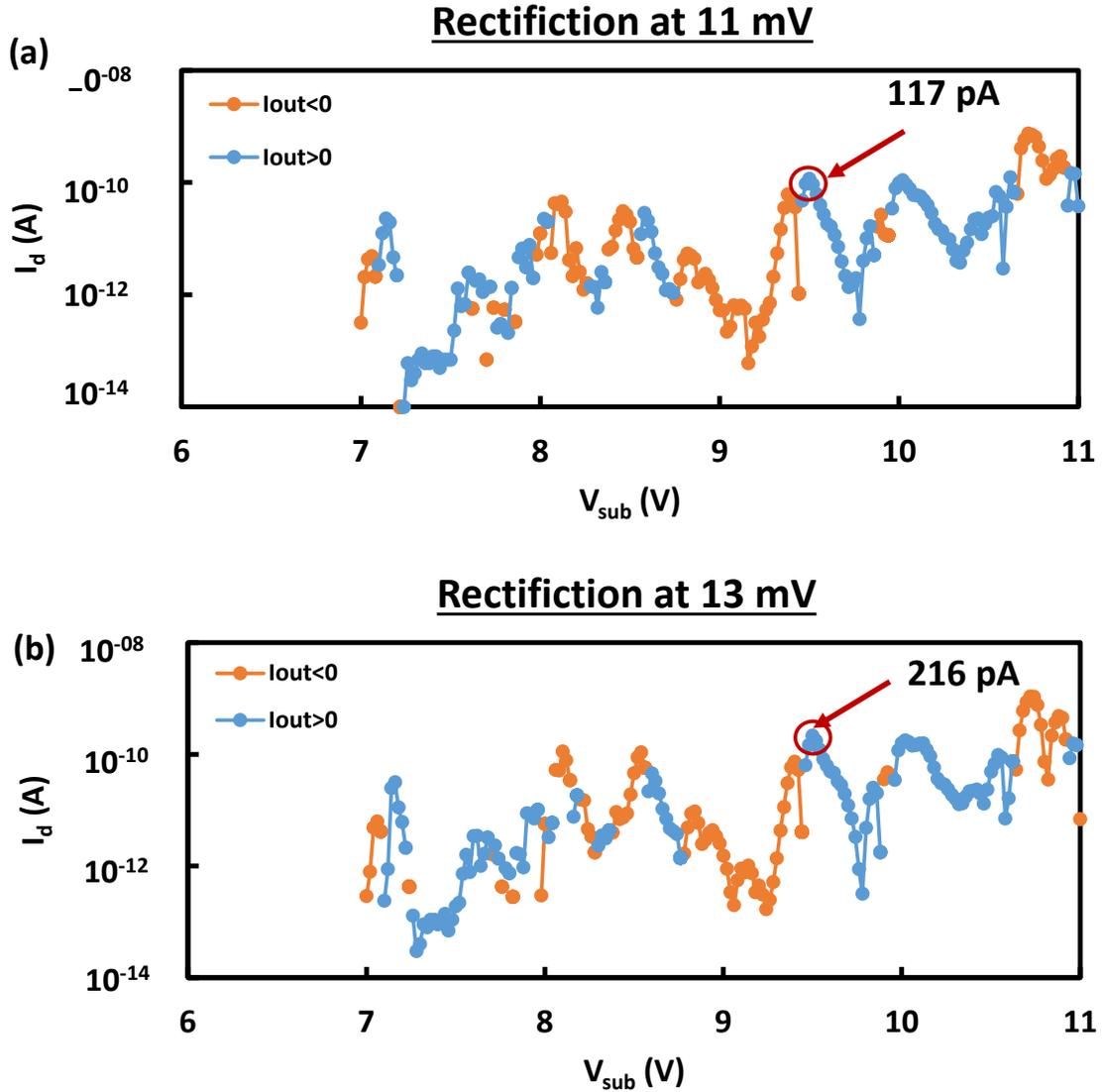
Fig. 3.22: Rectified current  $I_d$  as a function of substrate voltage  $V_{sub}$  at AC signal 1 MHz and amplitude (a) 11 mV and (b) 13 mV
