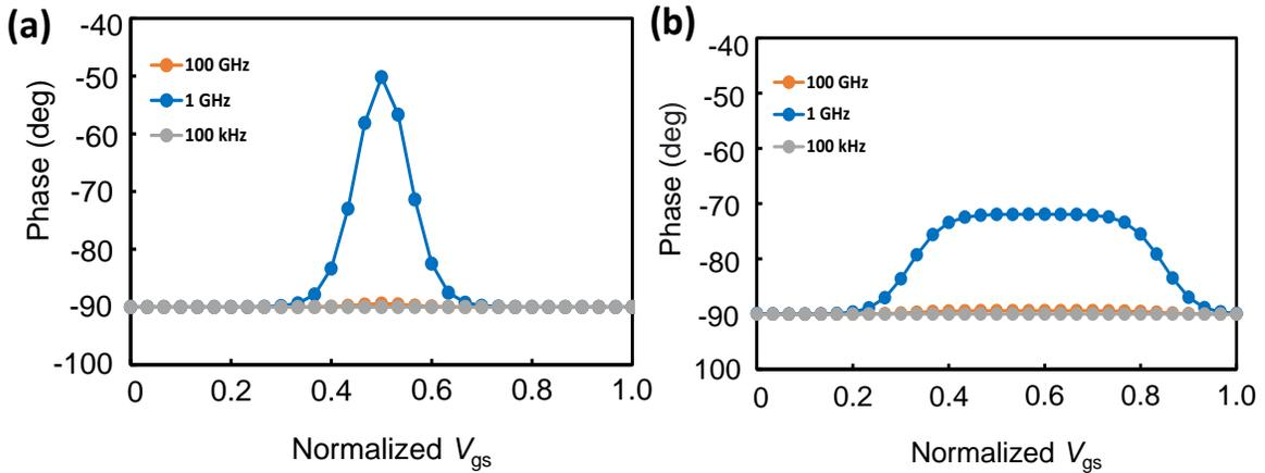
Fig. 2.14: Phase of the gate current with respect to the applied sinusoidal voltage in the circuit for  $C_{gg}$  evaluation [Fig. 2.11(a)] as a function of normalized gate voltage at drain voltages (a)  $V_{ds} = 0.534$  mV [0.01] and (b) 26.7 mV [0.5] and temperature  $T = 15.5$  K [0.05].
