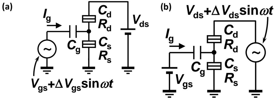
Fig. 2.11 Circuit diagrams for the measurement of (a)  $C_{gg}$  and (b)  $C_{gd}$ .
