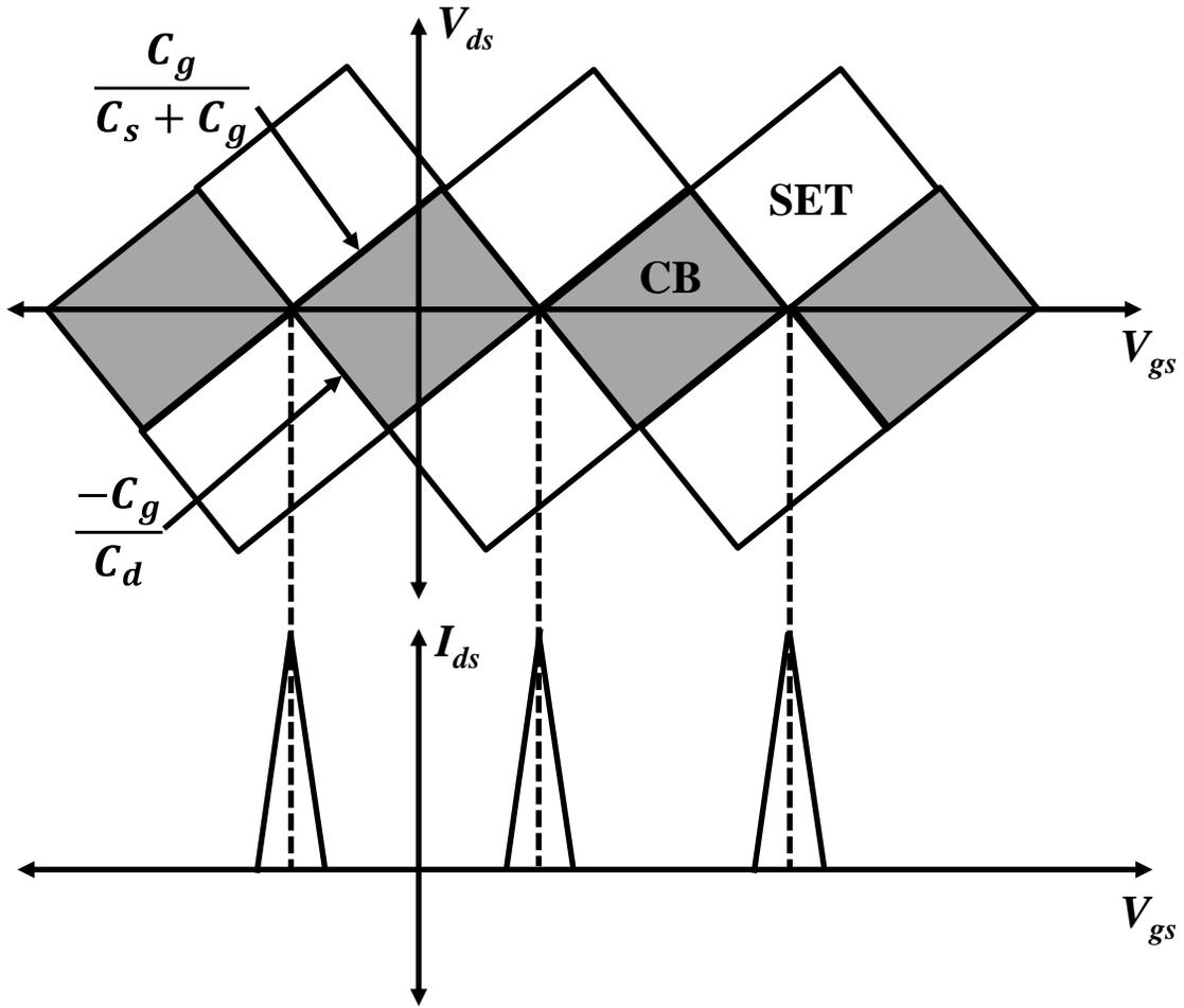
Fig. 2: Coulomb blockade boundary and corresponding drain current
