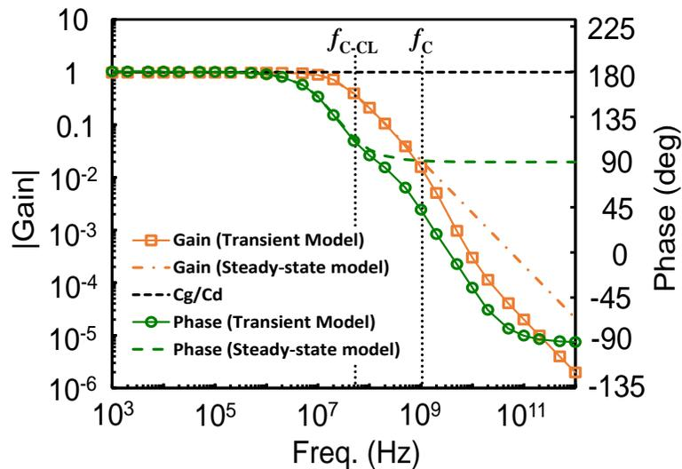
Fig. 2.22: Frequency response of the SET inverting amplifier with a load capacitor  $C_L=30$  aF ( $10C_\Sigma$ ) operating at a drain current  $I_d = 26.4$  pA, gate voltage  $V_{gs} = 53.4$  mV [0.33] (center of the descending side of the CD) and  $T = 15.5$  K [0.05].
