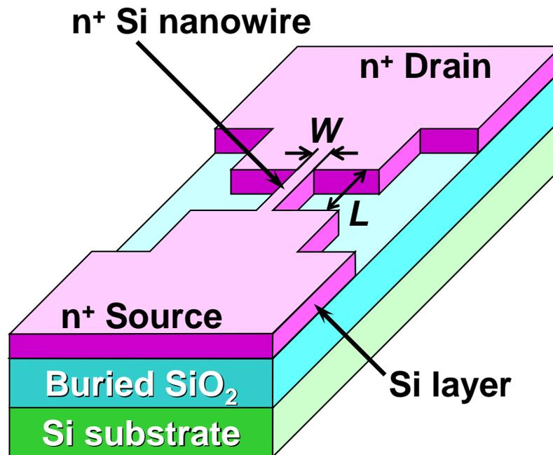
Fig. 3.11: Heavily doped silicon nanowire-based SET
