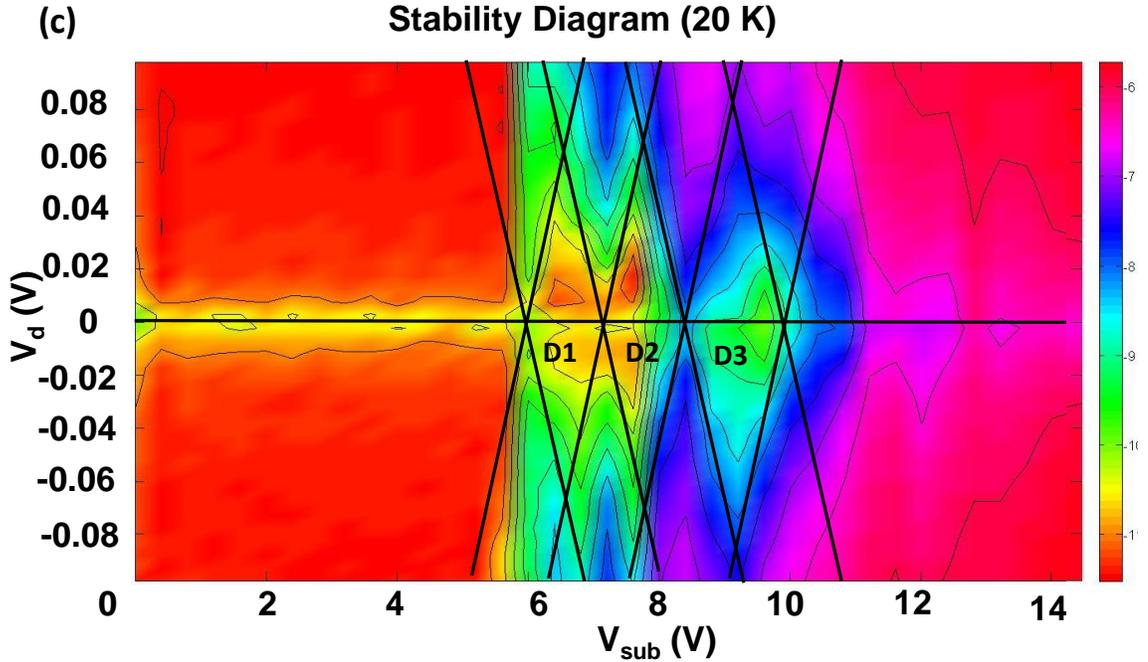
Fig. 3.21: (a)  $I_d$ - $V_{sub}$  (b)  $V_d$ - $V_{sub}$  and (c) Stability diagram of SET (L:1500 ; W: 30 nm)
