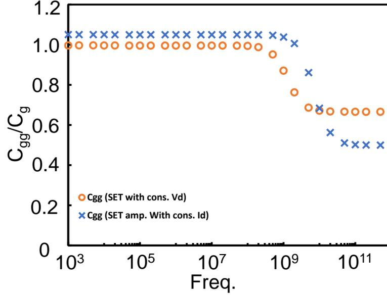
Fig. 2.20: SET input capacitance  $C_{gg}$  as a function of frequency at gate voltage  $V_{gs} = 53.4$  mV and temperature  $T = 15.5$  K [0.05]
