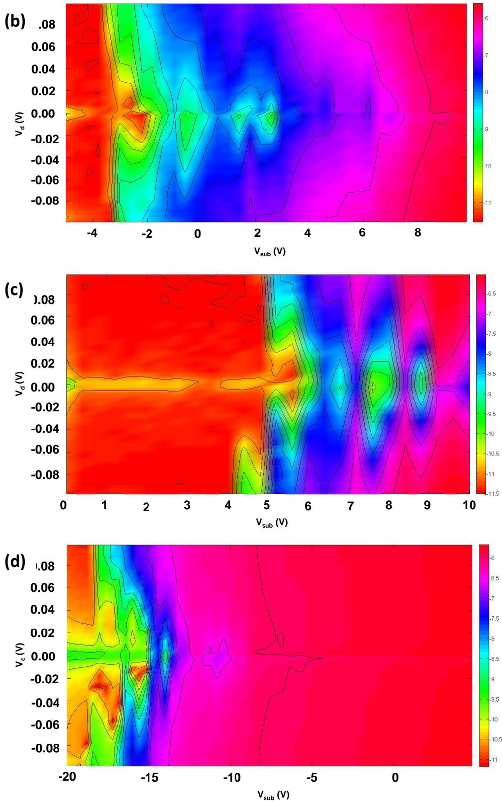
Fig. 3.20: Stability diagram of (a) #37a, L:500 nm, W:30 nm, D:0 (b) #30a, L:1000 nm, W:40 nm, D:1 (c) #44b, L:1500 nm, W:30 nm, D:2 and (d) #23c, L:3000 nm, W:50 nm, D:11
