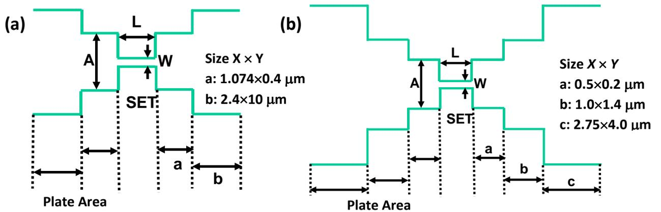
Fig. 3.6: Schematic diagram of heavily doped Si SETs channel (a) fabricated at SU (b) fabricated at HU. Note that each section  $a$ ,  $b$  or  $c$  is further divided into 10 subsections to properly simulate the distributed circuit characteristics [8].
