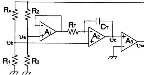
Fig. 1. A linear resistance-to-frequency converter: Basic configuration.
