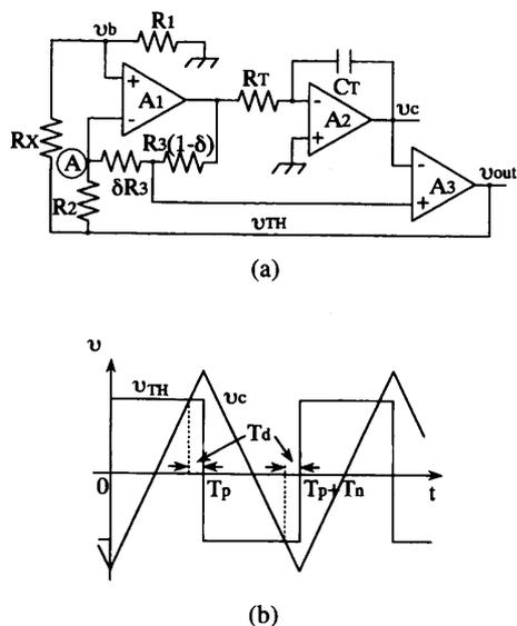
Fig. 3. (a) The circuit diagram of the delay-compensated resistance-to-frequency converter, (b) Voltage waveforms at the input terminals of comparator  $A_3$ .
