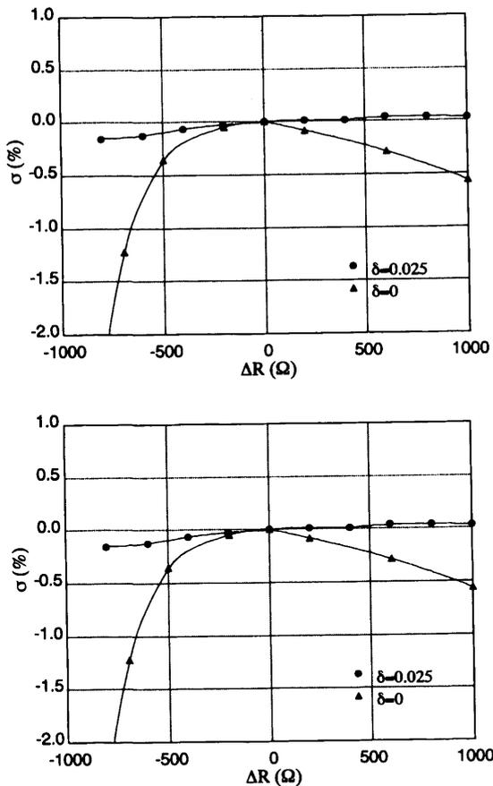
Fig. 5. The nonlinear error  $\sigma$  of the prototype converter with ( $\delta = 0.025$ ) and without ( $\delta = 0$ ) the delay compensation.
