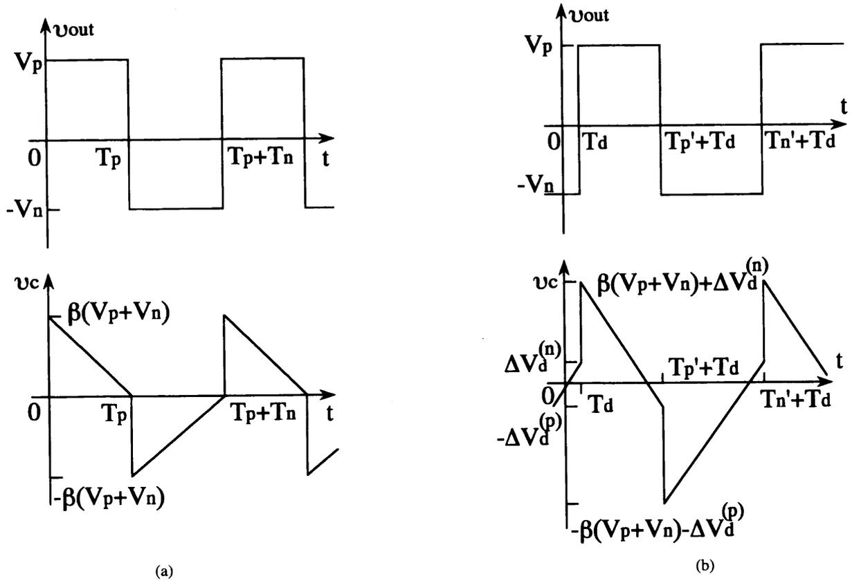
Fig. 2. Voltage waveforms in Fig. 1, (a) when op-amps are ideal and (b) when the zero-crossing detector has the response delay  $T_d$ .
