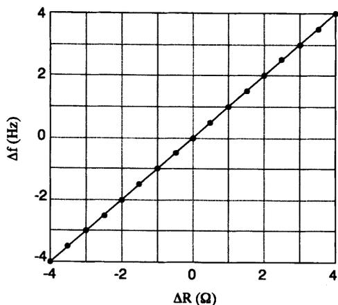
Fig. 4. The oscillation frequency change  $\Delta f$  of the prototype converter for the resistance change  $\Delta R$ .
