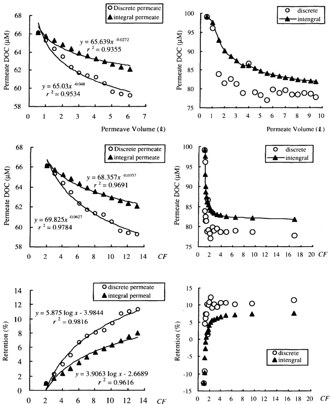
Fig. 2 Variations of the concentration of organic carbon in discrete permeate samples and the retention percentage with permeate volume and concentration factors increasing using natural seawater from Bora Bay.
