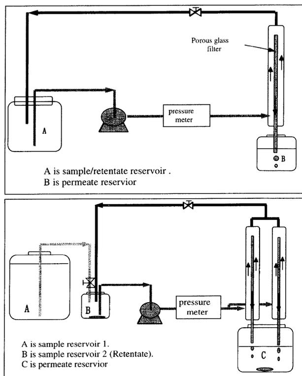
Fig. 1 Schematic of the cross-flow filtration systems used in this study. All joints, tubings and valves are made of Teflon.
