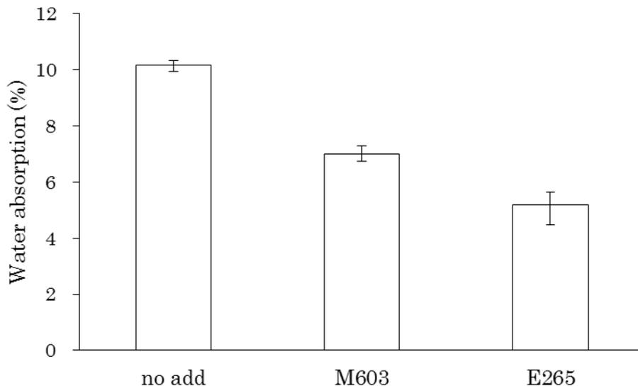
Fig.3 Effect of a coupling agent (MAPE) on water absorption
