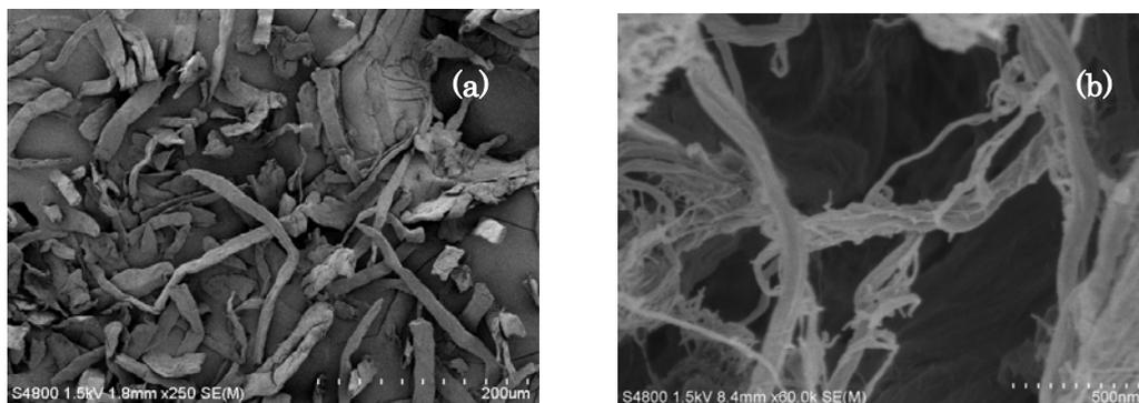
Fig.4 SEM photograph of the cellulose powder: (a) before ball milling and (b) after ball milling at 250rpm for 4 hours.
