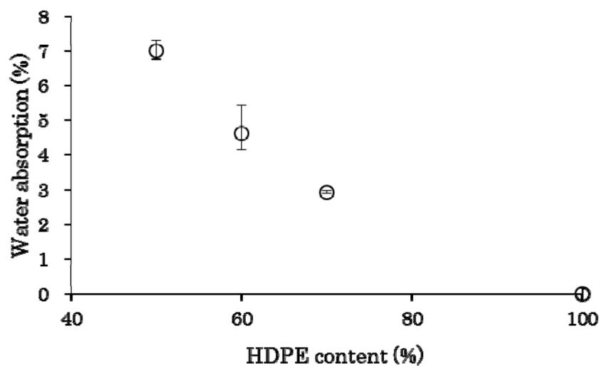
Fig.1 Effect of HDPE content on water absorption
