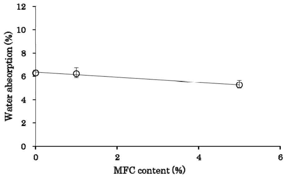
Fig.5 Effect of MFC content on water resistance of the mold
