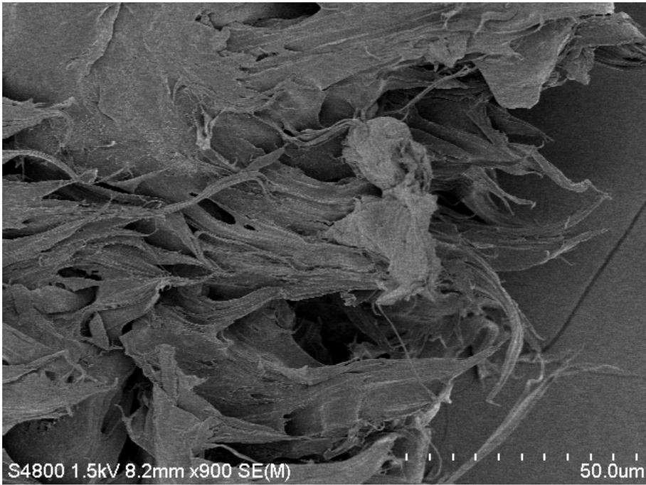
Fig.2 SEM photograph of the fracture surface of the No.2 composite (49% of HDPE content) after the tensile test
