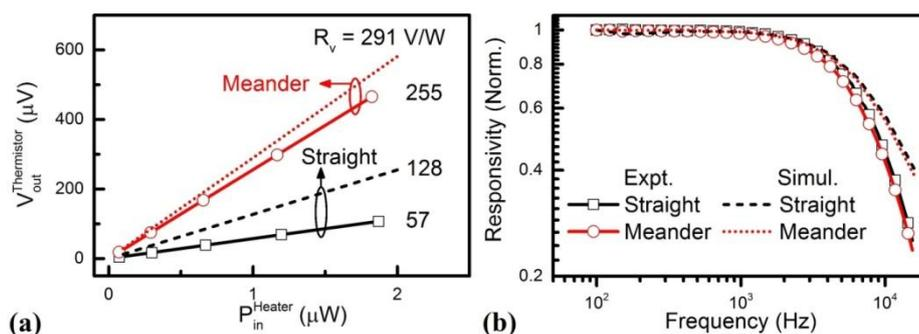
**Fig. 6. The experimental and simulated results of Ti microbolometer (a) Thermistor output versus heater input power for straight and meander shape thermistor at 100 Hz, and (b) frequency response of Ti microbolometer for straight and meander shape thermistor at 2  $\mu\text{W}$  input power. The symbol shows the experimental result, while dashed and dotted lines show simulated result.**
