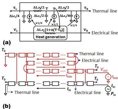
**Fig. 4. Electro-thermal (E-T) circuit for simulation (a) unit circuit, and (b) entire circuit for integrated thermistor and heater for meander shape thermistor.**
