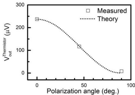
**Fig. 7. Thermistor signal of the room temperature THz antenna-coupled microbolometer responding to the 1 THz radiation as a function of the polarization angle of the radiation. The polarization angles of 0 and 90 degrees are on the E-plane and the H-plane, respectively. [Ref. 18]**
