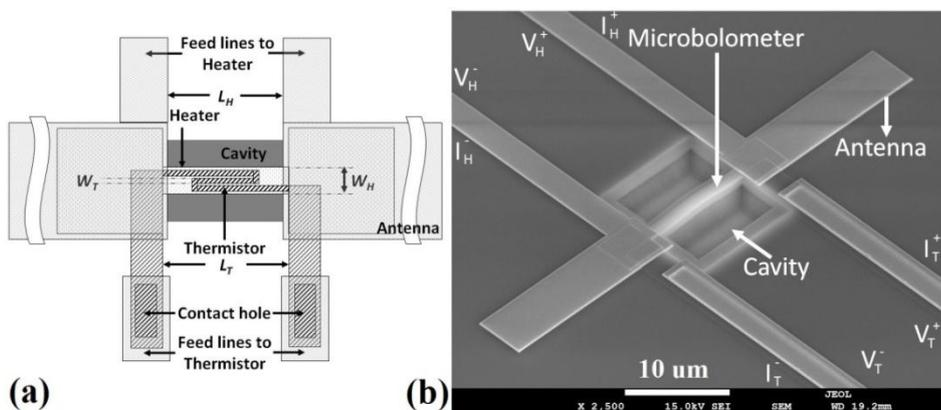
**Fig.2.**Antenna-coupled THz microbolometer. (a) Schematic diagram of the integrated thermistor/interlayer/heater are at the center of the half-wave dipole antenna, (b) SEM image of microbolometer fabricated by electron beam lithography. Here  $I_T^-$ ,  $I_T^+$  and  $V_T^-$ ,  $V_T^+$  are current and voltage terminals respectively for thermistor, whereas  $I_H^-$ ,  $I_H^+$  and  $V_H^-$ ,  $V_H^+$  are similar terminals for heater.
