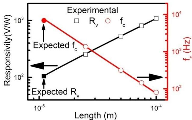
**Fig. 1.** Length dependence of responsivity ( $R_v$ ) and cutoff frequency ( $f_c$ ). Open square and circular symbols represent the  $R_v$  and  $f_c$  respectively while the closed square and circular symbols show the expected  $R_v$  and  $f_c$  respectively. Thickness and width of thermistor are 46 and 0.1  $\mu\text{m}$ , respectively, and those of heater are 96 and 1.24  $\mu\text{m}$ , respectively.
