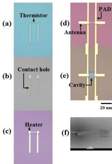
**Fig. 3. The fabrication steps of Ti microbolometer (a) thermistor pattern, (b) contact hole in SiO<sub>2</sub> interlayer, (c) heater integrated on thermistor, (d) Au-antenna and electrical pads, (e) cavity for thermal isolation of integrated thermistor and heater and (f) SEM image of meander shape thermistor.**
