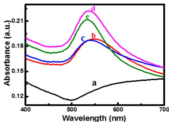
**Figure S1.** Ultraviolet-visible absorption spectroscopy of Au nanoparticle (NP) films deposited on polystyrene 96 well plates with different concentrations of HCOONa: (a) 100 mM; (b) 200 mM; (c) 300 mM; (d) 400 mM and (e) 500 mM.
