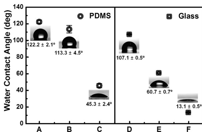
**Figure 3. Mechanistic study of Au NP deposition onto a substrate.** Static water contact angle ( $\theta_{st}$ ) values were measured on PDMS and glass with different treatments. Insets: digital images of water droplets (10  $\mu$ L in volume) placed onto each substrate.
