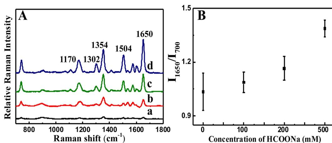
**Figure 4. Surface-enhanced Raman scattering of Au NP films deposited onto the PDMS substrate.** (A) SERS profiles of Au nanoparticle films deposited onto PDMS surfaces with (a) 0 mM, (b) 100 mM, (c) 200 mM and (d) 500 mM HCOONa. (B) The calibration curve of the Raman intensity versus HCOONa concentration. Error bars in (B) denote standard deviation ( $n = 3$ ).
