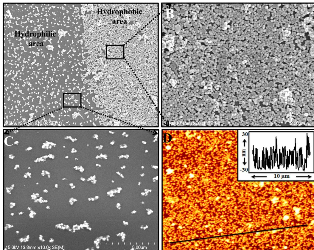
**Figure 2. Microscopic study of the films.** (A–C) SEM images of Au nanoparticles (NPs) deposited onto the surface of unmodified and modified PDMS substrates. (D) AFM image of Au NPs deposited onto the hydrophobic PDMS substrate (the inset shows the depth profile along the line).
