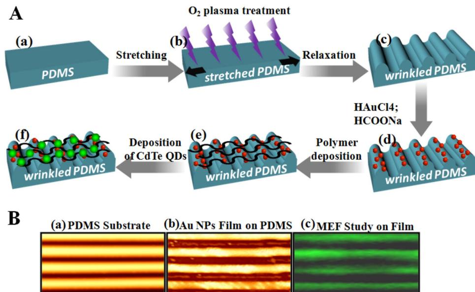
**Figure 5. Metal-enhanced fluorescence study on Au NP film.** (A) Schematic presentation of wrinkled PDMS substrate preparation (a–c), Au NP film fabrication on it (d) and CdTe QDs deposition using layer-by-layer method (e,f). (B) AFM image of bare wrinkled PDMS substrate (a), Au NP film formation on wrinkled PDMS substrate (b) and fluorescence microscopy image of Au NP film/QDs hybrid structure (c).
