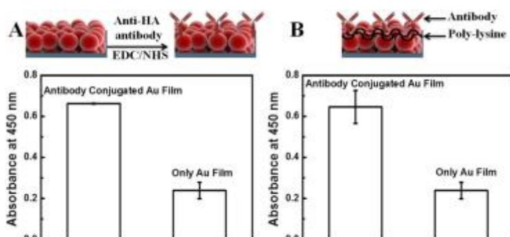
**Figure S9:** ELISA test of antibody binding to the film. Binding of the anti-HA (H1N1) Ab 66189 antibody to the nanostructured Au films using (A) EDC/NHS chemistry and (B) the layer-by-layer method (right).
