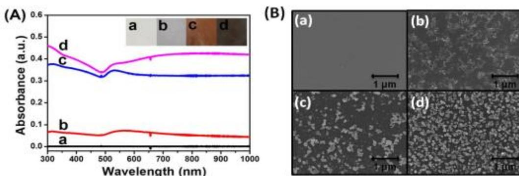
**Figure S2.** (A) UV-Vis absorption spectra and photographs of the Au NPs fabricated glass substrate using different concentration of HCOONa; a (0 mM), b (100 mM), c (200 mM), d (500 mM). Insets show the color of the glass substrates after deposition. (B) Scanning electron microscope images of nanostructured films on glass, which were deposited with solutions containing (a) 0 mM, (b) 100 mM, (c) 200 mM, and (d) 500 mM HCOONa.
