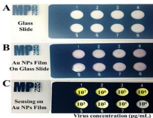
**Figure S11:** A photographic image of sensing on glass slide. (A) Cleaned glass slide; (B) Au NPs film on glass slide and (C) color developments on glass slide during sensing experiment.
