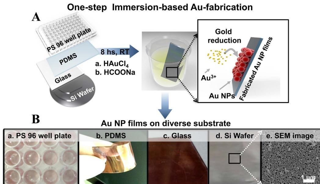
**Figure 1.** Presentation of the single-step, immersion-based fabrication of Au NP films on diverse substrates. (A) Procedure for the fabrication of the Au NP films. (B) Photographic images of Au NP films deposited on 96-well polystyrene plate (a), PDMS (b), glass (c), silicon wafers (d) and SEM image of densely packed Au NPs on silicon substrate (e).
