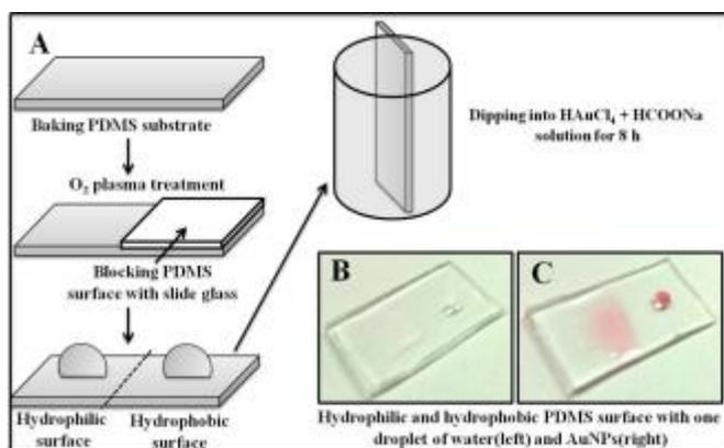
**Figure S3:** PDMS substrate preparation and its surface modification.
