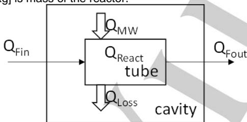
Figure 2 Heat energy flow around a reactor.
