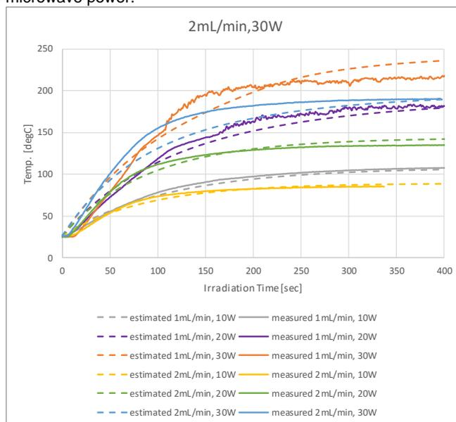
Figure 6 Measured and estimated temperature profile using optimized parameter  $a$  for microwave irradiation.
