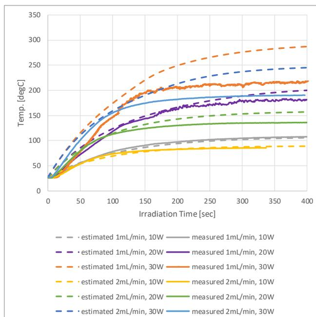
Figure 5 Measured and estimated temperature profile for microwave irradiation.
