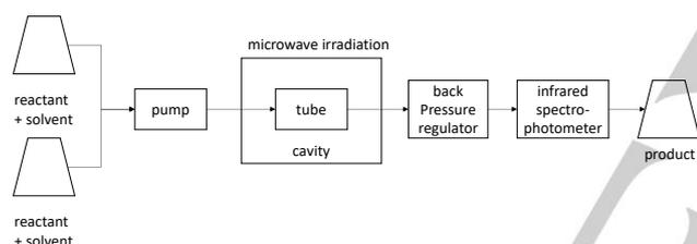
Figure 1 Schematic of a flow reactor heated by microwave irradiation.
