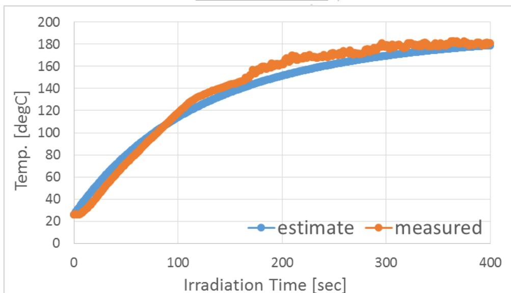
**Abstract:** Flow reactors heated by microwave irradiation attract attention. The reactors are suitable for difficult synthesis processes due to rapid heating and cooling, and easy pressurization. In order to predict the quality of the product, it is appropriate to estimate the outlet conditions of the reactor. In this paper, the outlet temperature of the flow direction is estimated by using the flow condition and dynamic thermal energy balance of the reactor.
