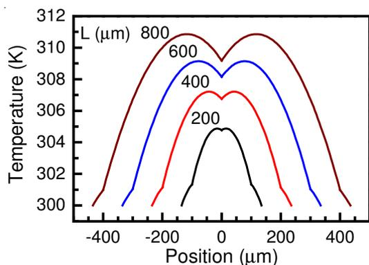
Fig. 4. Temperature distribution along the heater length predicted by electro-thermal circuit simulation
