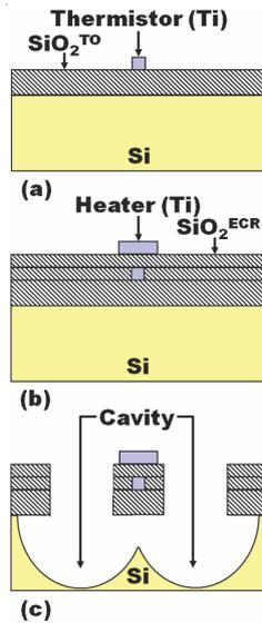
Fig. 1. Ti microbolometer fabrication steps along YY' cross-section. (a) Thermistor pattern, (b) heater pattern on top of ECR SiO<sub>2</sub> interlayer deposited on thermistor, and (c) suspended microbolometer structure above the cavity in Si substrate
