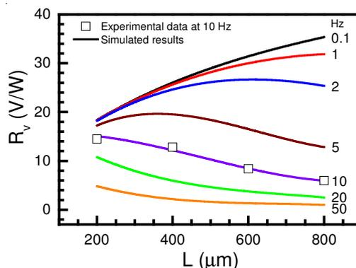
Fig. 6. The experimental and simulated responsivity of Ti microbolometer as function of heater length. The symbols show the experimental result, while solid lines show simulated results at different frequencies
