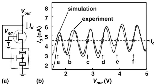
**Fig. 5** Schematic diagram (a) and  $I_d$ - $V_{out}$  characteristics (b) of the two-terminal multippeak NDR device. The experimental data (solid line) [7] were obtained at a  $V_{gg}$  of 1.08 V. Simulated characteristics obtained by SPICE are also shown (dotted curve). Stability points (a~f) expected for a current load of 4.5 nA are indicated by circles.
