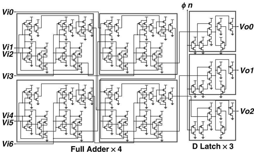
Fig. 13 Conventional 7-3 counter designed only with MOSFETs. Transistor count is 194. Power consumption is estimated to be  $360\mu\text{W}$  at  $V_{dd} = 3.3\text{ V}$  and  $f = 100\text{ MHz}$  for  $0.35\text{-}\mu\text{m}$  devices (equivalently  $110\mu\text{W}$  in the  $0.25\text{-}\mu\text{m}$  generation).
