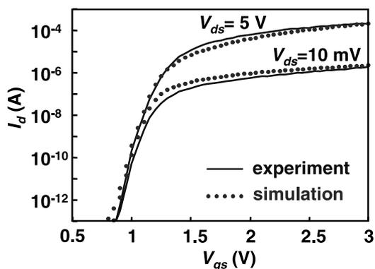
**Fig. 4**  $I_d$ - $V_{gs}$  characteristics of a MOSFET fabricated on the same SOI wafer as the SET, measured at 27K (solid line) [4]. Characteristics simulated by the BSIM3 model [11] are also shown (dotted line). The channel width and length and gate oxide thickness are 12  $\mu$ m, 14  $\mu$ m, and 90 nm, respectively. The measured threshold voltage  $V_{th}$ , corresponding to  $I_d = 4.5$  nA and  $V_{ds} = 3$  V, is 1.07 V.
