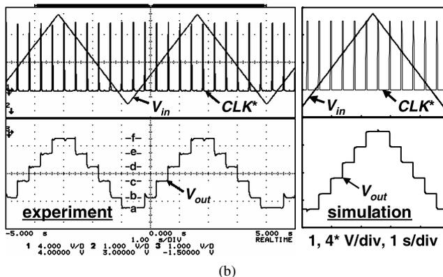
**Fig. 6** Schematic diagram (a) and experimental [4] and simulated waveforms (b) of the quantizer.
