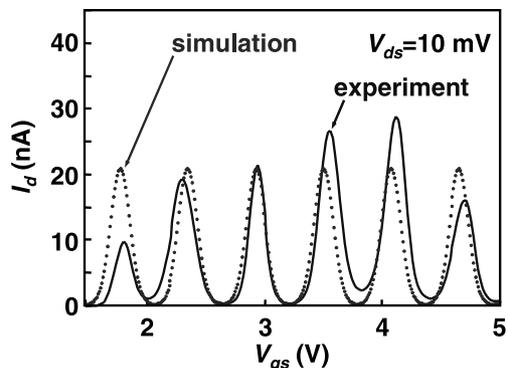
**Fig. 3**  $I_d$ - $V_{gs}$  characteristics of the fabricated SET, measured at 27K (solid line) [4]. Simulated characteristics with the analytical SET model are also shown (dotted line).
