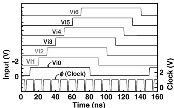
**Fig. 9** Waveforms of inputs  $V_{i0} \sim V_{i6}$  and clock  $\phi$ . High and low levels of the inputs are  $-1.12$  and  $-0.12$  V, respectively. The clock levels are  $1.05$  and  $-0.5$  V, respectively. The data are shifted for clarity.
