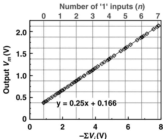
**Fig. 8** Simulated input-output characteristics of the inverting adder.  $C_i = 100$  aF,  $C_f = 400$  aF,  $V_L = -0.12$  V,  $V_H = -1.12$  V,  $\phi_n = 1.05$  V,  $V_{dd} = 2.5$  V,  $V_{ss} = -0.85$  V, and  $I_o = 230$  nA are assumed.
