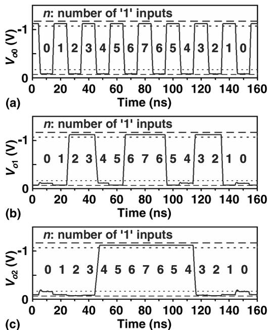
Fig. 12 Simulated output waveforms for literal0 (a), literal1 (b) and literal2 (c) corresponding to the inputs in Fig. 9.  $V_{ddn} = -1.12\text{ V}$ ,  $V_{ggn} = -1.04\text{ V}$ ,  $I_{on} = -170\text{ nA}$ ,  $C_m = 100\text{ aF}$ , and a capacitive load of 100 aF for each output (not shown in Fig. 7) are assumed. Typical output '1' and '0' voltages are  $-1.12$  and  $-0.12\text{ V}$ , respectively. Dashed and dotted lines indicate 110% and 90% of the typical amplitude, respectively.
