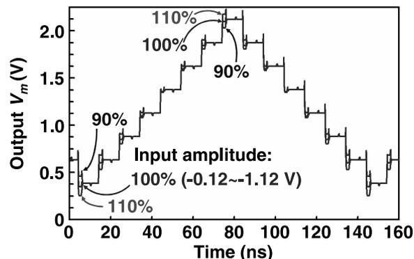
**Fig. 10** Simulated output waveforms of the latched quantizer for three combinations of input ‘1’ and ‘0’ levels,  $-1.12 \sim -0.12$  V (100%),  $-1.07 \sim -0.17$  V (90%), and  $-1.17 \sim -0.07$  V (110%). Input amplitude variation of  $\pm 10\%$  is cancelled by the quantizer and does not affect the output.
