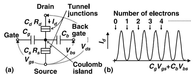
**Fig. 1** Equivalent circuit (a) and transfer characteristics (b) of a SET. The number of electrons in the Coulomb island is controlled by the gate and the backgate via gate capacitor  $C_g$  and backgate capacitor  $C_b$ , respectively. Drain current  $I_d$  flows periodically with respect to gate voltages  $V_{gs}$ ,  $V_{bs}$ , where the number of electrons is half-integer.
