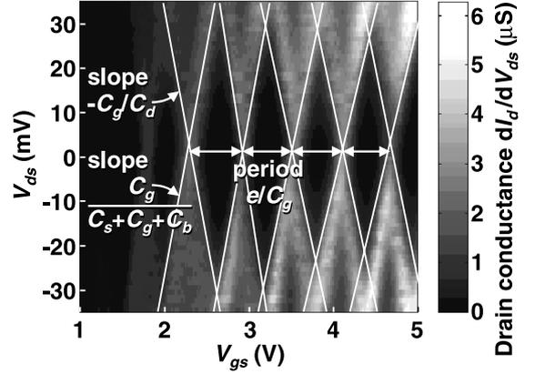
**Fig. 2** A Coulomb diamond (drain conductance contour) plot of a SET fabricated by the PADOX process, measured at 27K [4]. Capacitance parameters,  $C_g$ ,  $C_b$ ,  $C_s$  and  $C_d$ , are extracted from the slopes and the period.
