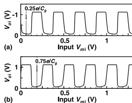
**Fig. 11** Simulated input-output characteristics of the SET periodic literals operated with negative (a) and positive (b) supply voltages. Input voltages for the first ‘0’ output are shifted to  $0.25e/C_g$  and  $0.75e/C_g$ , respectively, due to the SET drain voltage  $|V_{ds(SET)}|$  of  $e/2C_g$ .
