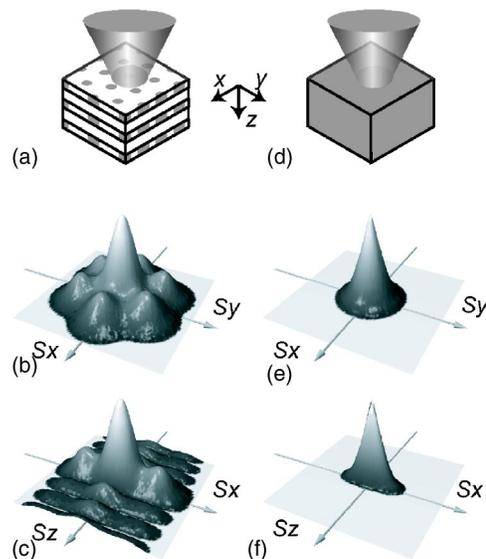
FIG. 1. Bit recording process and spatial frequency distribution of a recorded bit in structured as well as plain media. (a) Bit recording process in a structured medium. (b), (c) Spatial frequency distribution of a recorded bit in a structured medium along the  $S_x-S_y$  and  $S_x-S_z$  planes, respectively. (d) Recording process in a plain medium. (e), (f) Spatial frequency distribution of a recorded bit in a plain medium along the  $S_x-S_y$  and  $S_x-S_z$  planes, respectively.
