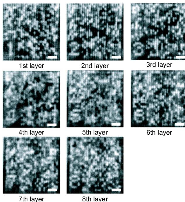
FIG. 3. View of recorded bit patterns in different layers of the 3D patterned medium. The bit interval in the transverse direction is  $0.5 \mu\text{m}$ . The spacing of neighboring recording layers is  $2.0 \mu\text{m}$ . Thus, a storage density of  $2.0 \text{ Tbits/cm}^3$  is achieved. The scale bars are  $2.0 \mu\text{m}$ .
