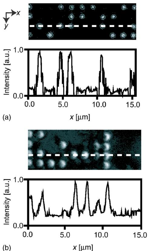
FIG. 4. Comparison of readout signals with a reflection-type confocal system from a (a) patterned medium and (b) plain medium.
