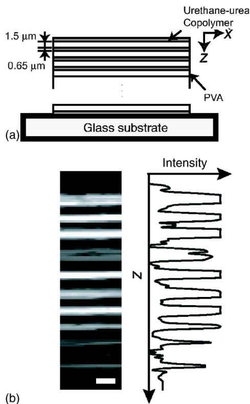
FIG. 2. (a) Structure of the multilayered recording medium. (b) Axial response of the multilayered medium observed with a reflection-type confocal microscope. The scale bar is  $2.0 \mu\text{m}$ .
