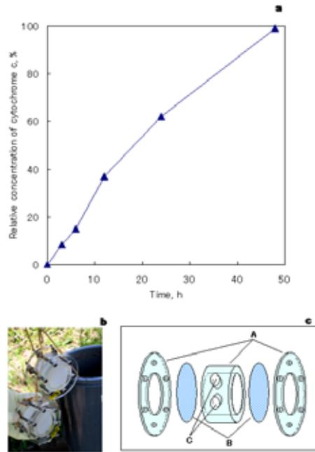
Fig. 1. Concentration of cytochrome c inside the diffusion chamber relative to the concentration outside the chamber (a). Photo of the diffusion chamber (b). Structure of the diffusion chamber (c), A: acrylic parts; B: 0.2 μm Nuclepore filters; C: sampling holes.
