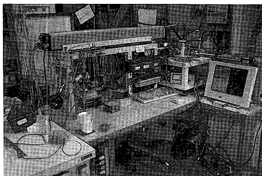
Fig. 2 Photograph showing the general setup of the vacuum line and laser. The pneumatic valves are controlled by the computer with the labVIEW software. Laser generating system is placed on top of the line by means of steel frame with adjustable bolts to fix the distance between the outlet lens and the sample holder.
