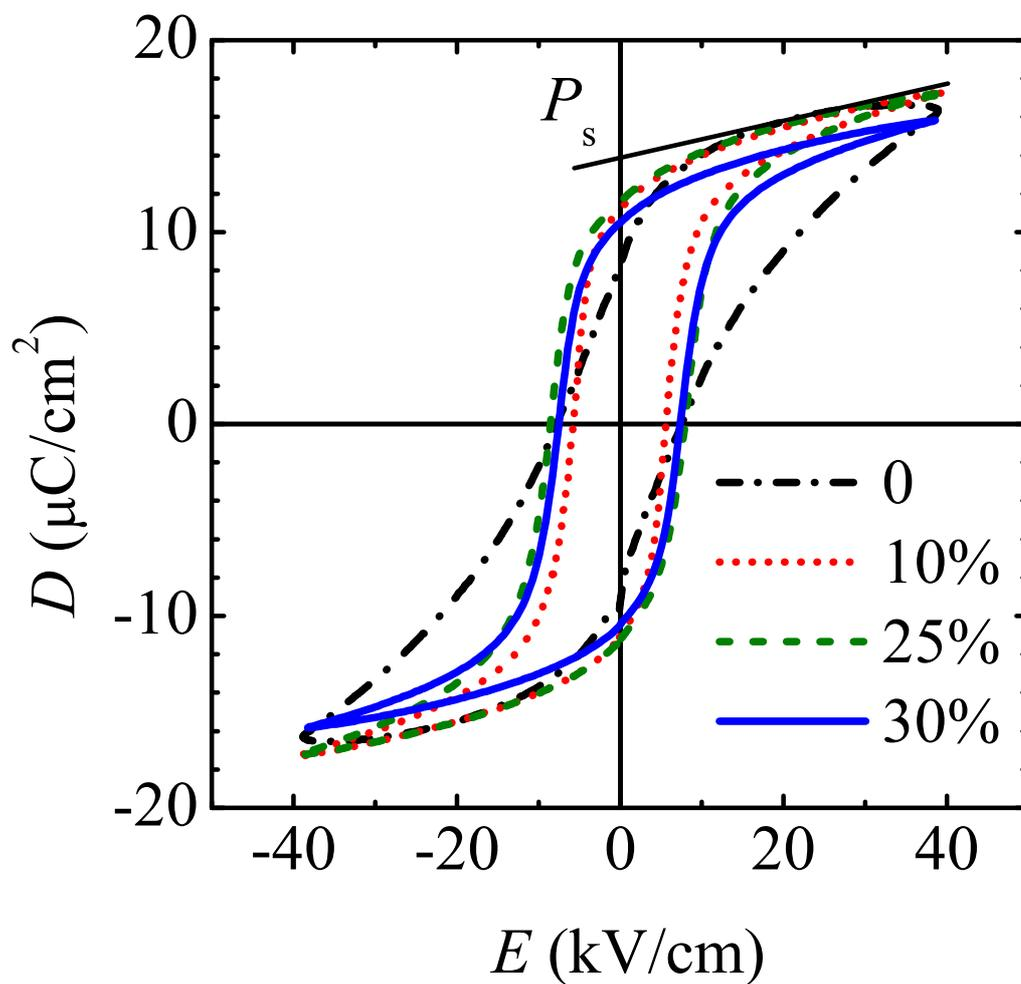
**Figure 3.** (Color Online) Typical  $D - E$  loops observed at room temperature for the ceramic samples of  $\text{Ba}_{1-x}\text{Ca}_x\text{TiO}_3$ .
