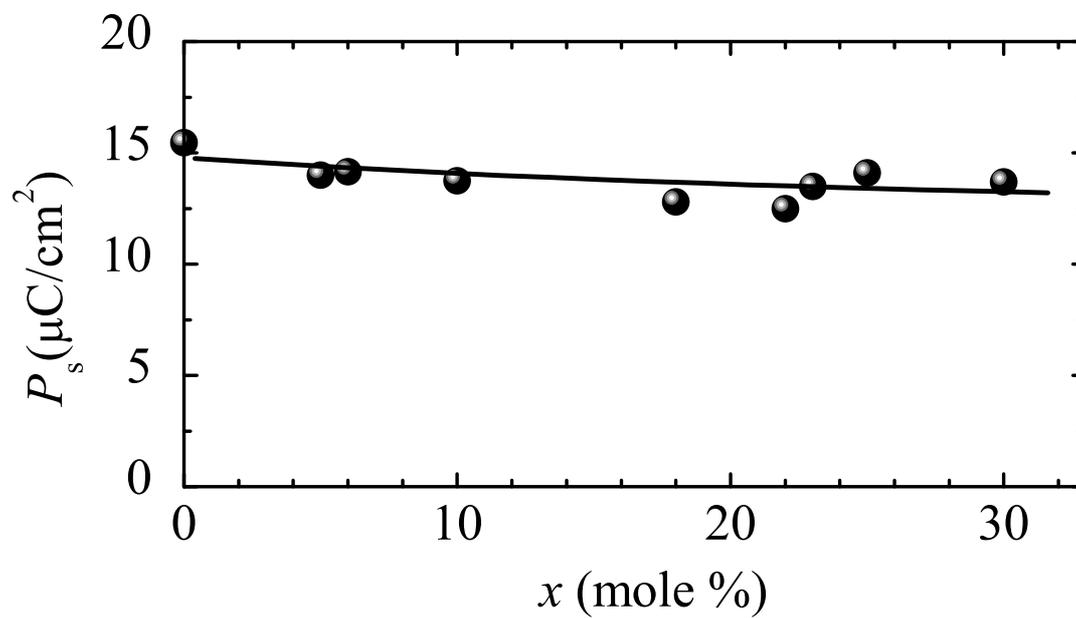
**Figure 4.** Compositional dependence of the saturation polarization of  $\text{Ba}_{1-x}\text{Ca}_x\text{TiO}_3$  ceramic samples.
