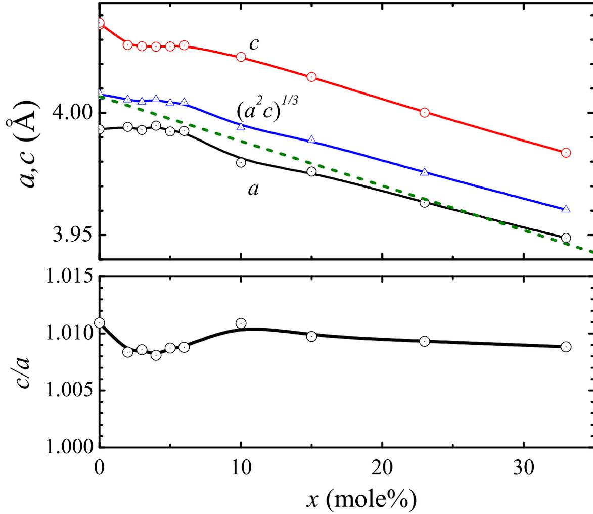
**Figure 2.** (Color Online) Compositional dependence of the lattice constant (upper panel) and tetragonality (lower panel) in  $\text{Ba}_{1-x}\text{Ca}_x\text{TiO}_3$ . The triangles show the variation of observed perovskite parameters  $(a^2c)^{1/2}$  in comparison with that predicted by the Vegard's law (dashed line).
