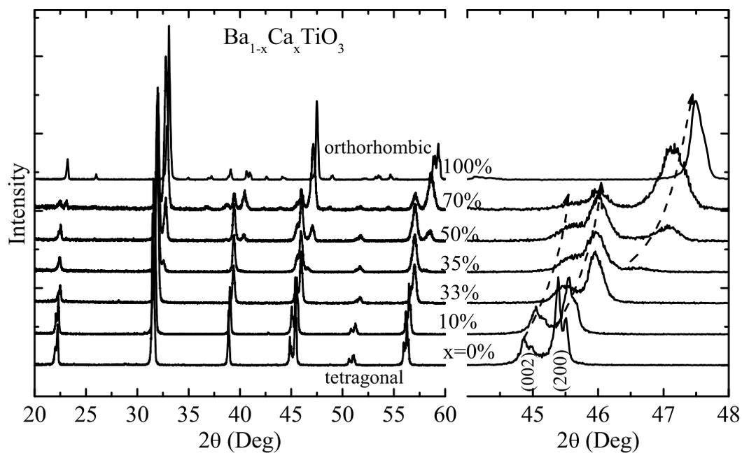
**Figure 1.** Phase evolution in the  $\text{BaTiO}_3\text{-CaTiO}_3$  system viewed from the powder X-ray diffractions at room temperature. The right panel shows an enlarged view of the variation of the diffractions in the  $2\theta$  range of  $44 - 48^\circ$ .
