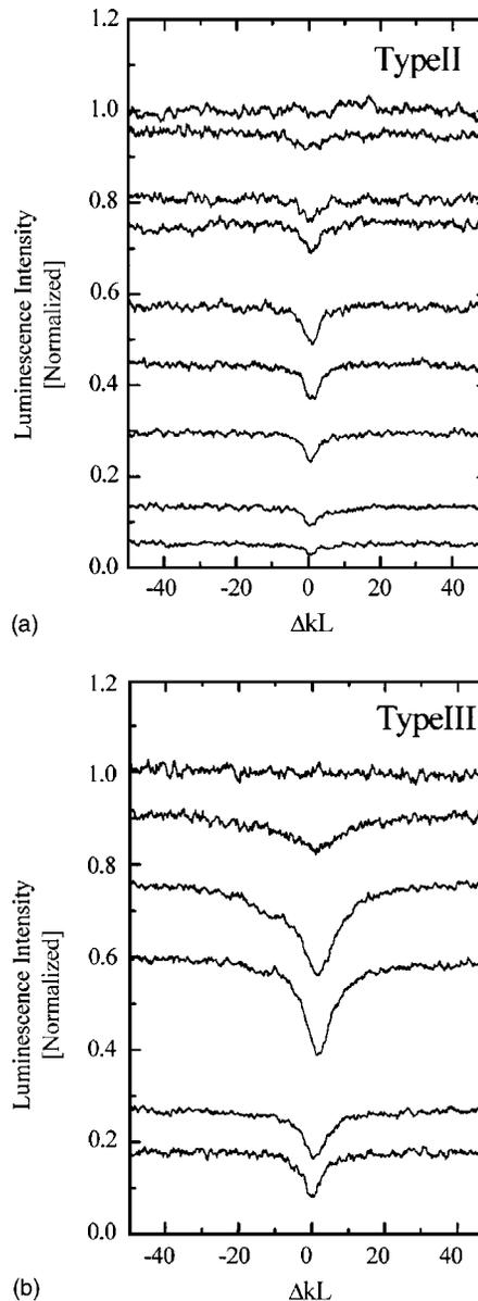
FIG. 8. (a) The luminescence intensity as a function of  $\Delta kL$  in the type II sample in the reflection geometry. From the top to the bottom,  $T_w = 0, 10, 20, 40, 80, 160, 320, 600, 1260 \text{ s}$ , respectively. (b) The luminescence intensity as a function of  $\Delta kL$  in the type III sample in the reflection geometry. From the top to the bottom,  $T_w = 0, 30, 330, 1350, 3900, 7500 \text{ s}$ , respectively.
