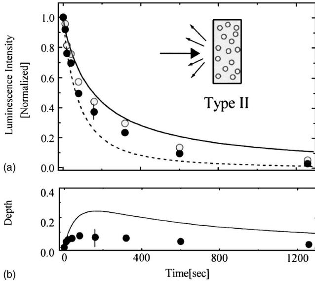
FIG. 9. Experimental results for the time development of the hole burning in the type II sample in the reflection geometry. (a) Solid and open circles represent  $\tilde{H}(\Delta k=0)$  and  $\tilde{H}(\Delta k=\infty)$ , respectively. The dashed and solid lines are calculated curves on the basis of Eqs. (24) and (23). (b) The solid circles represent the hole depth. The inset in (a) shows a schematic illustration of the type II sample.
