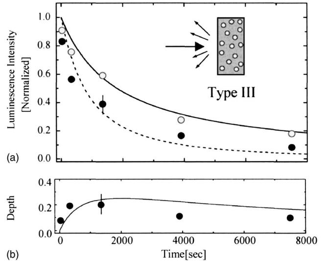
FIG. 10. Experimental results for the time development of the hole burning in the type III sample in the reflection geometry. (a) Solid circles and open circles represent  $\tilde{H}(\Delta k=0)$  and  $\tilde{H}(\Delta k=\infty)$ , respectively. The solid and dashed lines are guides for the eyes. The inset in (a) is a schematic illustration of the type III sample. (b) The solid circles represent the hole depth.
