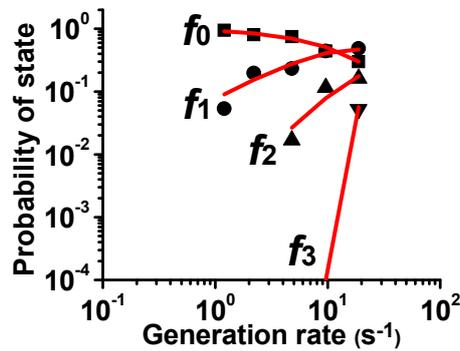
Fig. 6 (Color online) Probability of state obtained from Fig. 5 as a function of generation rate. States  $f_0, f_1, f_2$  and  $f_3$  correspond to the number of trapped holes of 0, 1, 2, and 3, respectively.
