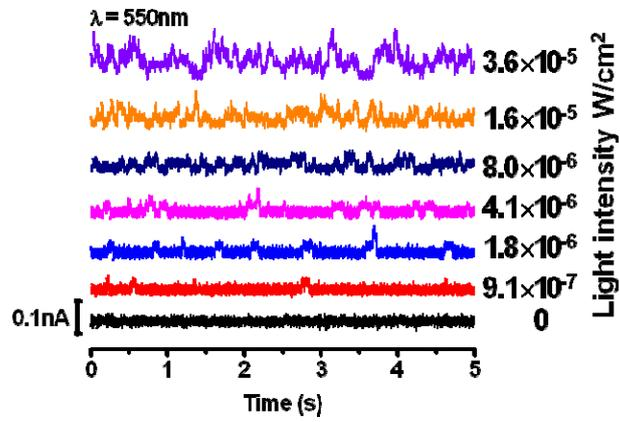
Fig. 3 (Color online) Drain current waveforms at 300 K for different levels of light intensity at a wavelength of 550 nm. Each waveform is shifted for clarity. Base line current is about 1nA.  $V_D$ ,  $V_{LG}$  and  $V_{SUB}$  are 0.05, -1, and 1V, respectively.
