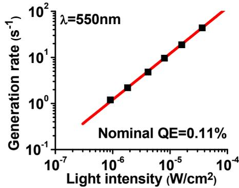
Fig. 4 (Color online) Pulse generation rate vs. incident light intensity. Slope of the fitting line is one.
