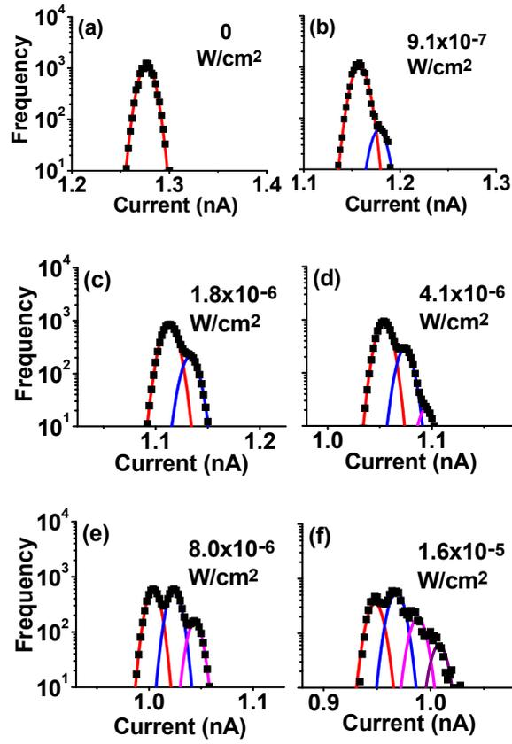
Fig. 5 (Color online) Histograms of digitized drain currents corresponding to Fig. 3. 1st, 2nd, 3rd and 4th peaks correspond to the number of trapped holes of 0, 1, 2, and 3, respectively. Data acquisition time period and time step are 5 s and 488  $\mu$ s, respectively, and 10,240 (=5 s/ 488  $\mu$ s) data points (current values) are classified into bins with a width of 2 pA.
