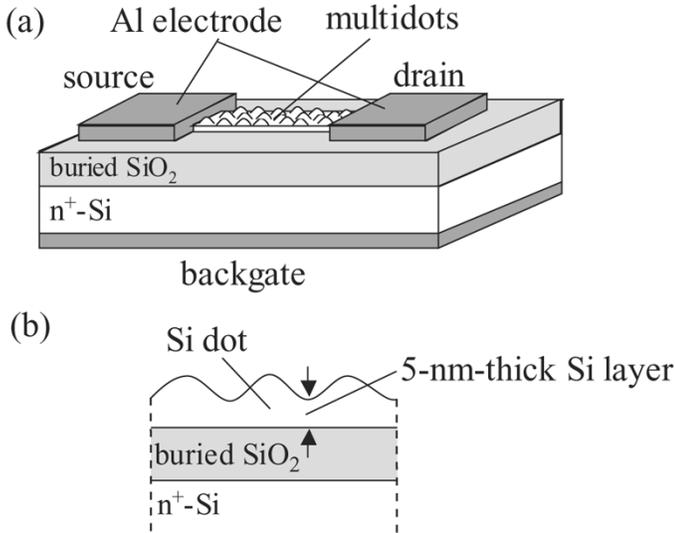
Fig. 2. Schematic view of Si SET device. (b) Cross-sectional view of the Si channel.
