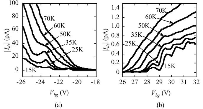
Fig. 6. Temperature dependence of  $I_{ds}$  at fixed  $V_{ds} = -15$  mV for (a) SHD and (b) SED conditions.
