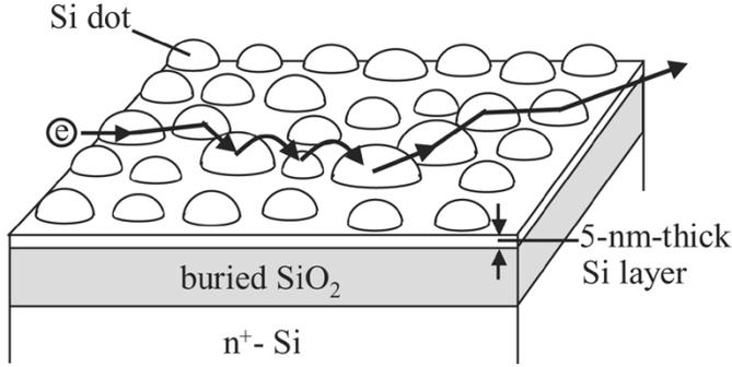
Fig. 4. Single-hole (electron) percolation path.
