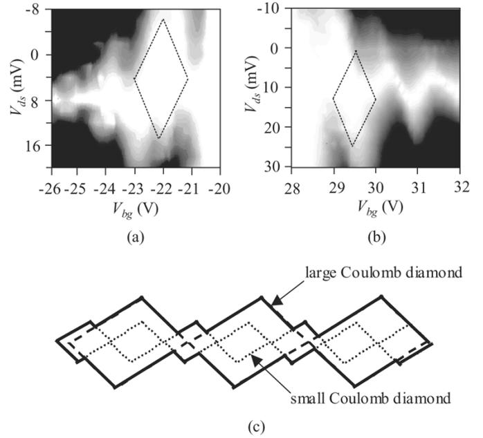
Fig. 5. Contour plot of the  $|I_{ds}|$  versus  $V_{bg}$  and drain-source voltage ( $V_{ds}$ ) for (a) SHD and (b) SED conditions. (c) Coulomb diamond diagram of two single-hole (electron) transistors connected in series.
