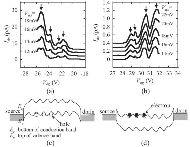
Fig. 3. Drain-source current ( $I_{ds}$ ) versus backgate voltage ( $V_{bg}$ ) of the (a) SHD and (b) SED characteristics at 15 K. The curves are shifted vertically by (a) 2 pA and (b) 0.1 pA, respectively, for clarity.
