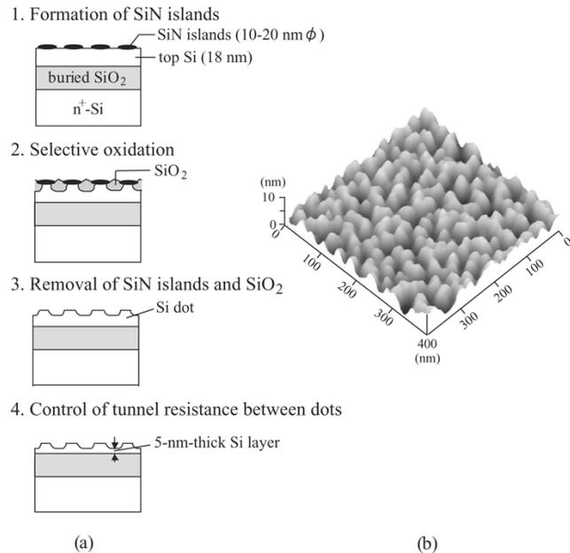
Fig. 1. (a) Fabrication steps of Si multidots. (b) AFM image of the fabricated dots.
