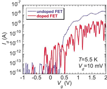
FIG. 4. (Color online) Experimental dc  $I_d$ - $V_g$  characteristics for a reference undoped-channel FET (dotted curve) and for a FET having the same dimensions but the channel moderately doped with phosphorus (solid curve).
