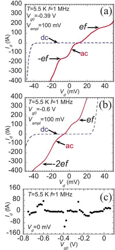
FIG. 5. (Color online) [(a) and (b)]  $I_d$ - $V_d$  characteristics measured under dc operation (dashed curves) and ac operation (solid curves) for the doped-channel FET for offset gate voltages of  $-0.39$  and  $-0.6$  V, respectively. Small plateaus aligned around  $\pm nef$  current levels can be noticed in both cases. (c)  $I_d$  at  $V_d=0$  V under ac operation as a function of gate offset voltage  $V_{g0}$ .
