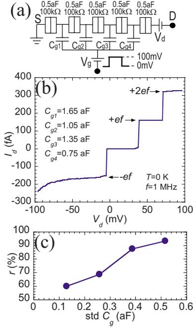
FIG. 1. (Color online) (a) Equivalent circuit of typically investigated 1D arrays. (b) Example of ac  $I_d$ - $V_d$  characteristics for uniform junction capacitances and resistances. Current plateaus can be observed at  $nef$  levels. (c) Effect of gate capacitance dispersion on quantized electron transfer. Rate  $r$  is defined as the number ratio of gate capacitance arrangements exhibiting quantized electron-transfer plateaus to all 16 investigated configurations.
