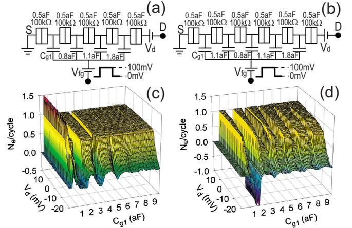
FIG. 3. (Color online) [(a) and (b)] Equivalent circuits for 1D arrays with four and five quantum dots, respectively, and parameters chosen for analysis. [(c) and (d)] Mesh plots of average number of electrons transferred between the electrodes per cycle ( $N_e/\text{cycle}$ ) as a function of source-drain bias  $V_d$  and source-side gate capacitance  $C_{g1}$  for the cases of (a) and (b), respectively.
