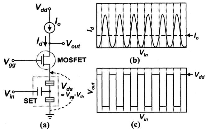
Fig. 1. (a) Schematic of the universal literal gate comprising a SET, a MOSFET and a constant-current (CC) load  $I_o$ . (b)  $I_d$ – $V_{in}$  characteristics, which are almost completely independent of  $V_{out}$  since the  $V_{ds}$  of the SET is kept nearly constant at  $V_{gg}$  minus  $V_{th}$ , the threshold voltage of the MOSFET. (c) Expected transfer ( $V_{in}$ – $V_{out}$ ) characteristics.
