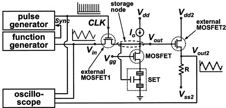
Fig. 9. Measurement setup for the quantizer proposed in Fig. 2(a). The central SET and MOSFET are on the same wafer. The external MOSFET1 is a transfer gate, and MOSFET2 is used as an FET probe to measure the  $V_{out}$  sustained by a small current ( $\sim nA$ ).
