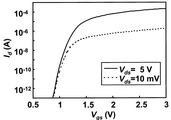
Fig. 6.  $I_d$ - $V_{gs}$  characteristics of a MOSFET fabricated on the same SOI wafer as the above SET, measured at 27 K. Effective channel width and length and gate oxide thickness are 12  $\mu\text{m}$ , 14  $\mu\text{m}$  and 90 nm, respectively. Threshold voltage  $V_{th}$ , corresponding to  $I_d = 4.5$  nA and  $V_{ds} = 3$  V, is 1.07 V, and transconductance  $G_m$  at  $V_{ds} = V_{gs} = 3$  V is 151  $\mu\text{S}$ .
