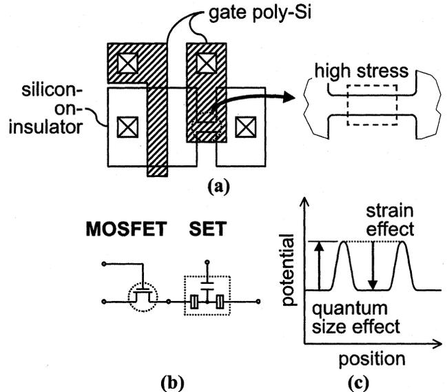
Fig. 3. (a) Possible layout of the integrated SET and MOSFET. (b) Circuit diagram corresponding to the layout above. (c) Potential profile along the length of the narrow wire, where a SET is created by pattern-dependent oxidation (PADOX) [20], [21]. Since areas outside the wire can readily be used for MOSFETs, PADOX is highly compatible with a CMOS process.
