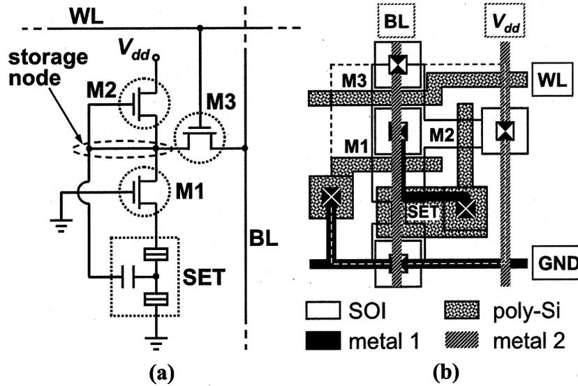
Fig. 14. Single-electron MV SRAM cell with two depletion-mode MOSFETs (M1 and M2) and one enhancement-mode MOSFET (M3). (b) An example of the SRAM layout. Metal-1 and 2 lines are drawn narrower for clarity. The unit cell area surrounded by the dashed line is  $31.1F^2$ , where  $F$  is half the minimum wiring pitch.
