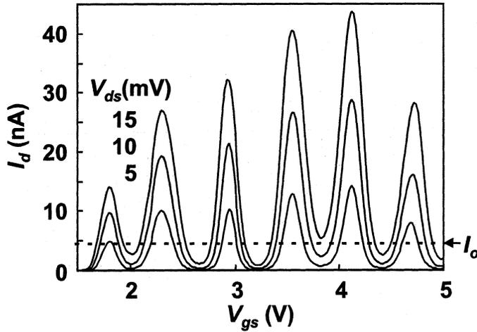
Fig. 4.  $I_d$ - $V_{gs}$  characteristics of a SET fabricated by the PADOX process, measured at 27 K.
