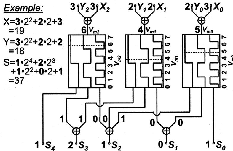
Fig. 13. A full adder for redundant positive-digit number representation PD2-3 [8] consisting of three ADC blocks without a quantizer, and linear sums ( $\oplus$ ). This adder is free from carry propagation, and is thus fast. By using the SET-MOSFET devices, multiple-valued logics of this kind can be made with half the number of elements in conventional implementation.
