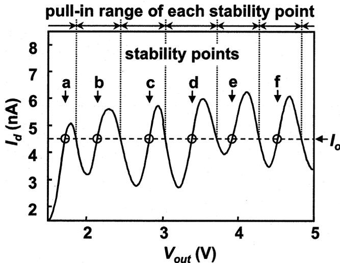
Fig. 8. Two-terminal  $I_d$ - $V_{out}$  characteristics of the SET-MOSFET device with the SET gate shorted to the MOSFET drain, measured at 1.08 V of  $V_{gg}$  [19]. Stability points (a~f) and the corresponding pull-in ranges expected for the current load of 4.5 nA are also shown.
