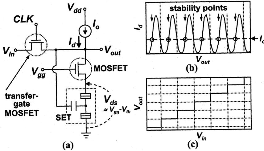
Fig. 2. (a) Schematic of the proposed quantizer (static memory). (b) Two-terminal  $I_d$ - $V_{out}$  characteristics of the SET-MOSFET device with the SET gate shorted to the MOSFET drain. (c) Expected transfer ( $V_{in}$ - $V_{out}$ ) characteristics.  $V_{in}$  is transferred to  $V_{out}$  through the transfer gate MOSFET and is quantized to a stability point after the gate is cut off.
