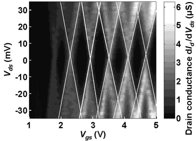
Fig. 5. Coulomb diamond plot of the SET shown in Fig. 4. From this figure, gate capacitance  $C_g$ , source capacitance  $C_s$ , drain capacitance  $C_d$  and tunnel resistance are calculated to be 0.27 aF, 2.7 aF, 2.7 aF and 80~220 k $\Omega$ , respectively.
