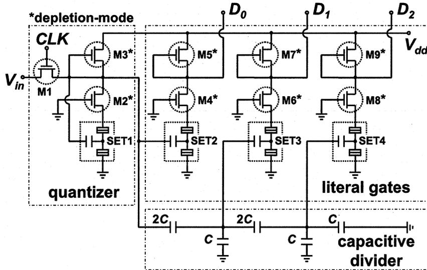
Fig. 12. The circuit diagram of the 3-bit ADC in Fig. 11. Depletion-mode MOSFETs, M2, M4, M6 and M8, keep the drain voltage of the SETs nearly constant at the absolute threshold voltage. Other depletion-mode MOSFETs, M3, M5, M7 and M9, serve as CC loads.
