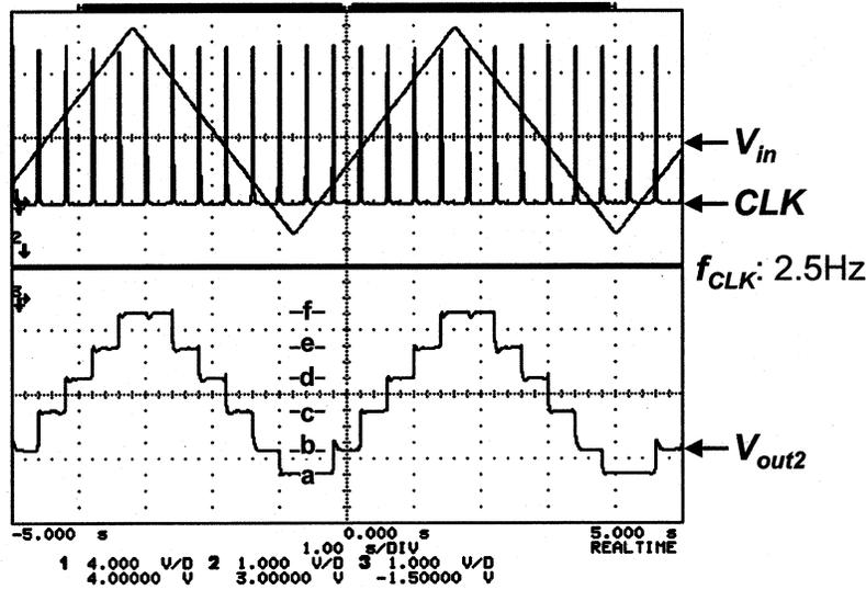
Fig. 10. Quantizer operation measured by the setup in Fig. 9, with  $V_{gg}$  of 1.08 V and a CC load of 4.5 nA. Operation speed is not limited by the intrinsic performance of the device, but by the large stray capacitance of 370 pF at  $V_{out}$ .
