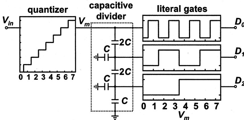
Fig. 11. A block diagram of a 3-bit flash ADC. A conventional  $n$ -bit flash ADC requires  $n^2 - 1$  components, whereas the SET ADC [24], [25] requires only  $n$ . This particular ADC with the quantizer at the front end and with the SET-MOSFET literal gates does not require comparators, latches, or ramp generators at each literal gate. Gray code is not necessary either.
