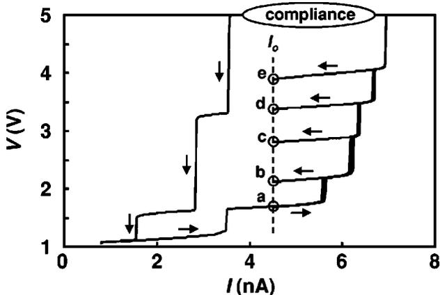
FIG. 3. Current sweep measurements of the NDR device in Fig. 2(b). The output voltage of the current source is limited by the compliance of 5 V.
