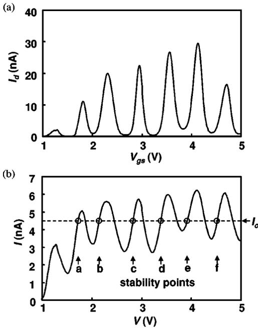
FIG. 2. (a)  $I_d$ - $V_{gs}$  characteristics of a SET for  $V_{ds}$  of 10 mV, measured at 27 K. (b)  $I$ - $V$  characteristics of the proposed NDR device for  $V_{gs}$  of 1.08 V measured at 27 K. Stability points (a-f) expected for a current load of 4.5 nA are indicated by circles. The SET was fabricated by the PADOX process (Refs. 9-11) together with the MOSFET on the same SOI wafer.
