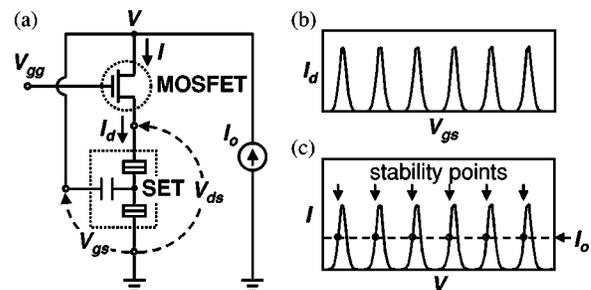
FIG. 1. (a) Schematic of the proposed multipeak NDR device comprising a SET and a MOSFET. A constant-current source  $I_o$  is connected for multiple-valued memory operation. (b) Typical  $I_d-V_{gs}$  (three-terminal) characteristics of a SET. (c) Expected  $I-V$  (two-terminal) characteristics of the SET-MOSFET device. Load line  $I_o$  and the corresponding stability points for memory operation are also shown.
