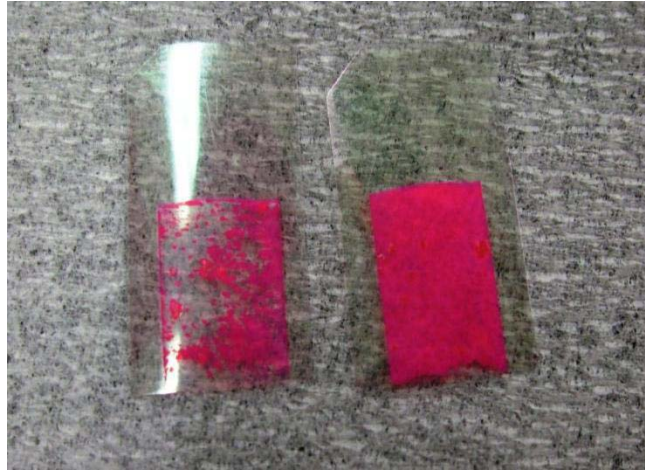
Fig. 3.3 State of peeling after hot press.
