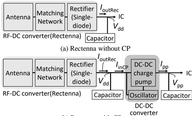
Fig. 1 Circuit block diagram
