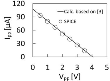
Fig. 4.  $V_{PP} - I_{PP}$  with  $V_{OP} = 1V$
