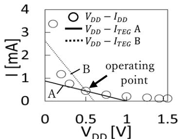
Fig. 2.  $V_{DD} - I_{DD}$  and  $V_{DD} - I_{TEG}$
