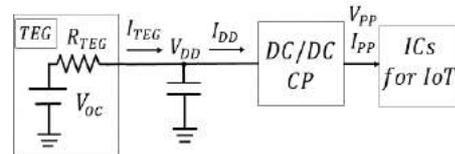
Fig. 1. Block diagram of IoT edge devices
