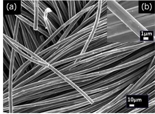
**Fig. 2** (a) SEM image of CAF and (b) its magnified image.
