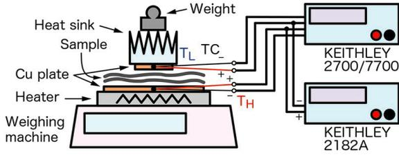
**Fig. 1** Schematic diagram of developed Seebeck coefficient measurement system.
