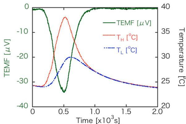
**Fig. 3** Time evolutions of TEMF and temperatures at hot  $T_H$  and cold  $T_L$  junctions for single CAF layer.
