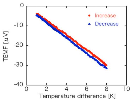
**Fig. 4** Relationship between TEMF and temperature difference for single CAF layer. “Increase” and “Decrease” correspond to the data collected from the range where the temperature difference is increasing and decreasing, respectively, in Fig. 3.
