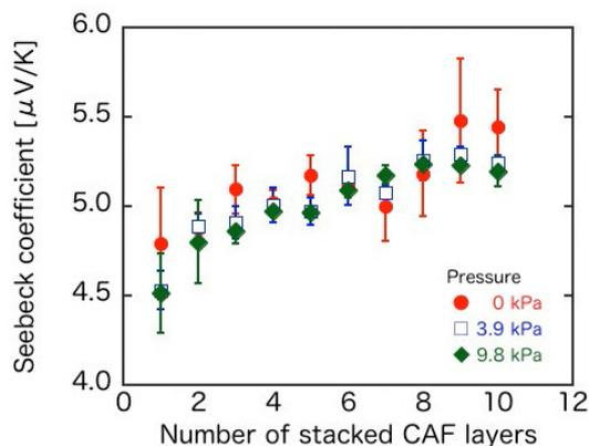
**Fig. 5** Relationship between Seebeck coefficient and the number of stacked CAF layers, as a parameter of extra pressure by weight. In the horizontal axis, 0 kPa corresponds to the pressure of heat sink only, 1.6 kPa.
