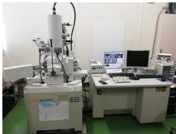
Figure 2. Scanning electron microscope (JEOL JSM 7001F)
