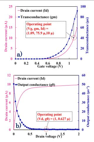
**Figure 5.** (a) Extraction of the transconductance (gm) from drain current vs. gate voltage characteristics; (b) extraction of the output conductance (go) from drain current vs. drain voltage characteristics. As an example, characteristics of the n-channel MOSFET with  $L=1~\mu m$  and  $W=5~\mu m$  are shown.  $V_d=1.00~V$  for (a), and  $V_g=1.09~V$  for (b).
