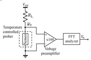
Figure 4. Circuit for noise measurement.
