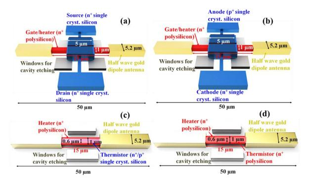
**Figure 1.** The structure of assumed antenna-coupled bolometers and its dimensions. (a) P or n-channel MOSFET bolometer, (b) pn-junction diode bolometer, (c)  $p^+$  or  $n^+$  single crystalline silicon resistive bolometer, and (d)  $n^+$  polycrystalline silicon resistive bolometer.
