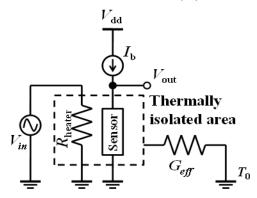
**Figure 2.** Equivalent circuit for responsivity  $(R_v)$  estimation.
