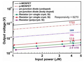
**Figure 7.** Estimated output voltage response of various bolometers for the heater input power. The ETF effect is not included in the lines for MOSFET and diode bolometers.
