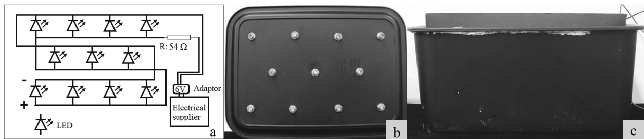
Figure 1: LED experimental box development, a. LED circuit in the experimental box composed of 11 LEDs with connecting to 54Ω resistor and the electrical wire for connecting to electrical supplier, b. the arrangement of LED bulbs on the cover of the experimental box, and c. outside view of experimental box
