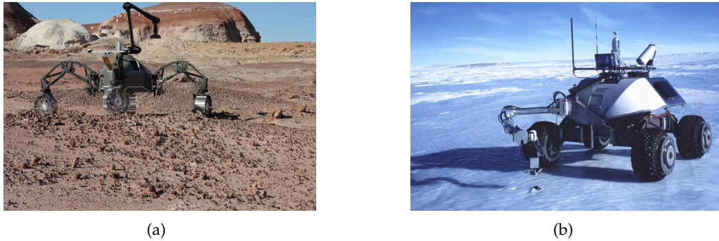
Figure 1.1: Typical outdoor terrains. (a) SherpaTT robot traversing undulating terrain abundantly covered with rocks (Cordes, Kirchner, and Babu, 2018); (b) Nomad robot searching for meteorites on an icy terrain in Antarctica (Wagner et al., 2001).
