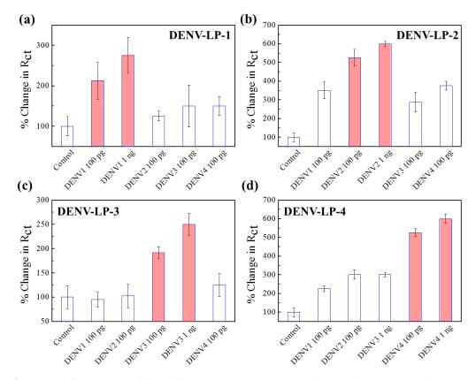
**Figure 5.** (**a**–**d**) Selectivity of four different DENV sensor electrodes with their corresponding target concentrations of 100 pg mL<sup>-1</sup> and 1 ng mL<sup>-1</sup> in the presence of other serotypes. Error bars represent the standard deviations of triple measurements.
