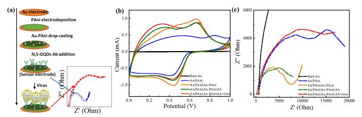
**Figure 1.** (a) Schematic diagram of the stepwise preparation of the sensor electrode, (b) cyclic voltammetry, and (c) electrochemical impedance results of Au | PAni | Au-PAni-Ab electrode before and after virus addition.
