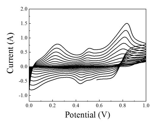
Figure S2. Electropolymerization of polyaniline on the bare Au electrode.
