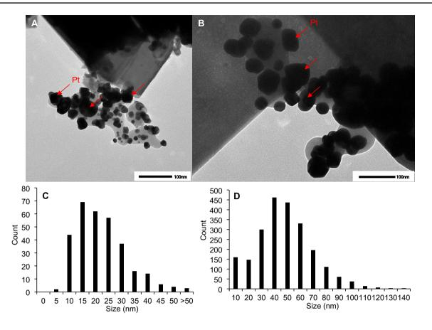
Fig. 5 TEM images of a Cs-Si-Pt-700-5 and b Cs-Si-Pt-800-5. The Pt particle size distributions in Cs-Si-Pt-700-5 and Cs-Si-Pt-800-5 are shown in c and d, respectively
