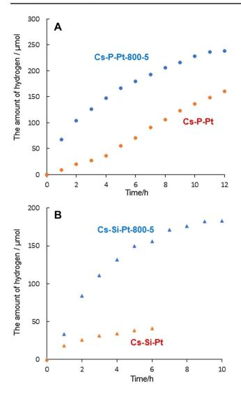
Fig. 6 Time course for hydrogen evolution catalyzed by a Cs-P-Pt-800-5 and Cs-P-Pt, and b Cs-Si-Pt-800-5 and Cs-Si-Pt. Reaction conditions: platinum catalyst (0.2  $\mu$ mol Pt), EY (2.5  $\mu$ mol), K-Si-Al (2.5  $\mu$ mol), TiO<sub>2</sub> (anatase:rutile=80:20) 50 mg, 100 mM aqueous TEOA solution (10 mL, pH 7), light irradiation ( $\lambda \ge 440$  nm), 25 °C
