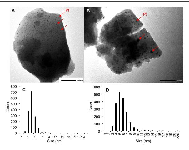
Fig. 4 TEM images of a Cs-P-Pt-700-5 and b Cs-P-Pt-800-5. The Pt particle size distributions of Pt Npts in Cs-P-Pt-700-5 and Cs-P-Pt-800-5 are shown in c and d, respectively
