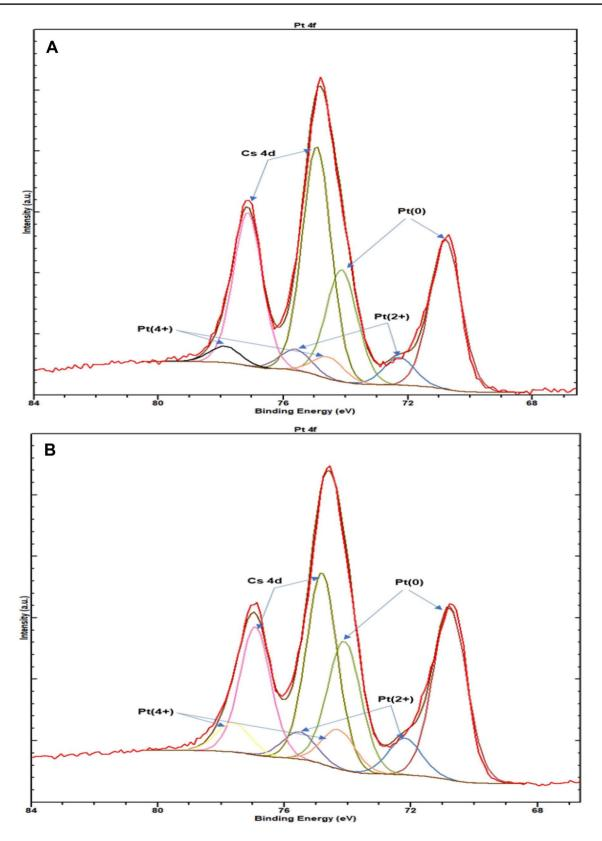
Fig. 3 Pt(4f) XPS spectra in the range 66.5–84 eV of a Cs-P-Pt-800-5 and b Cs-Si-Pt-800-5
