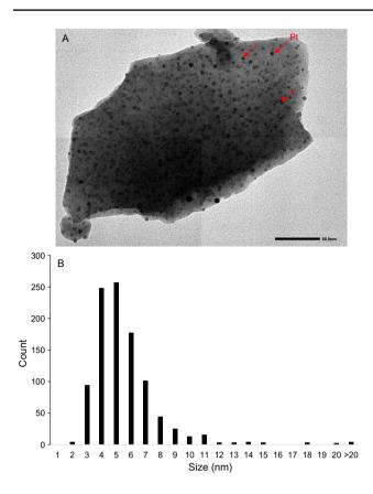
Fig. 8 a TEM image of Cs-P-Pt-800-5 after light irradiation, and b the size distribution of Pt Npts
