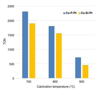
Fig. 7 A plot of TON after 6 h vs. calcination temperature of Cs-P-Pt and Cs-Si-Pt for hydrogen evolution from aqueous TEOA under visible light irradiation. Reaction conditions are shown in the caption of Fig. 6
