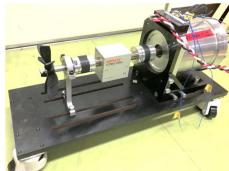
(b) Actual setup with propeller type fan.
