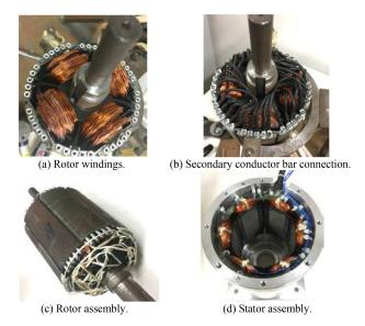
Fig. 8. Actual prototype machine.
