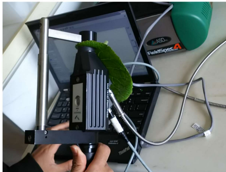
Figure 1. Measurements of the chlorophyll content of wasabi leaves using (a) the Colorcompass-LF and (b) the FieldSpec4.
