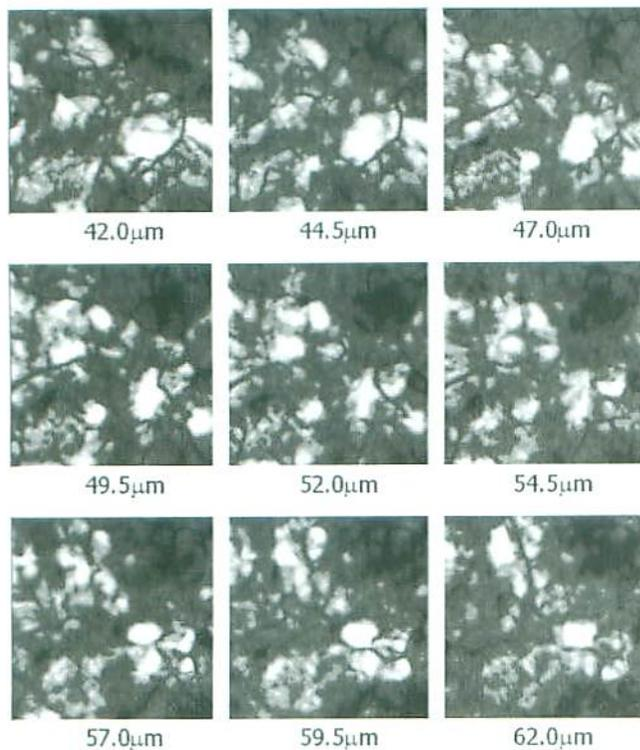
FIG. 2. (Color online) Cross-section luminescence intensity distributions image of polynomials ZnSe.
