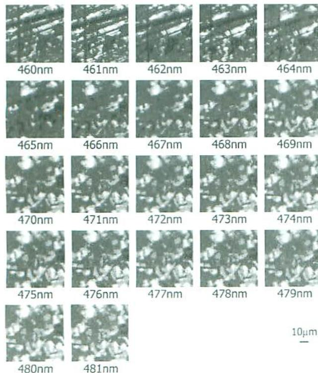
FIG. 3. (Color online) Spectral distribution images of polynomials ZnSe crystal filtered by monochromator.
