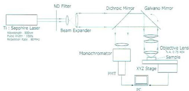
FIG. 1. (Color online) Experimental configuration on ZnSe using two-photon luminescence.
