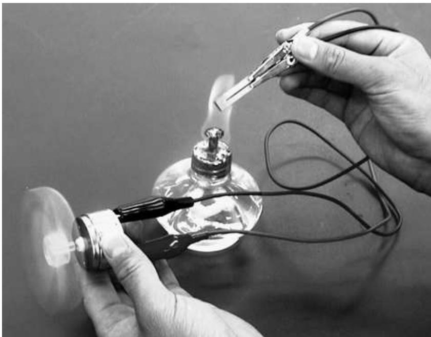
Fig. 4.9. Joined Si-Ge element with a slit heated by a frame.
