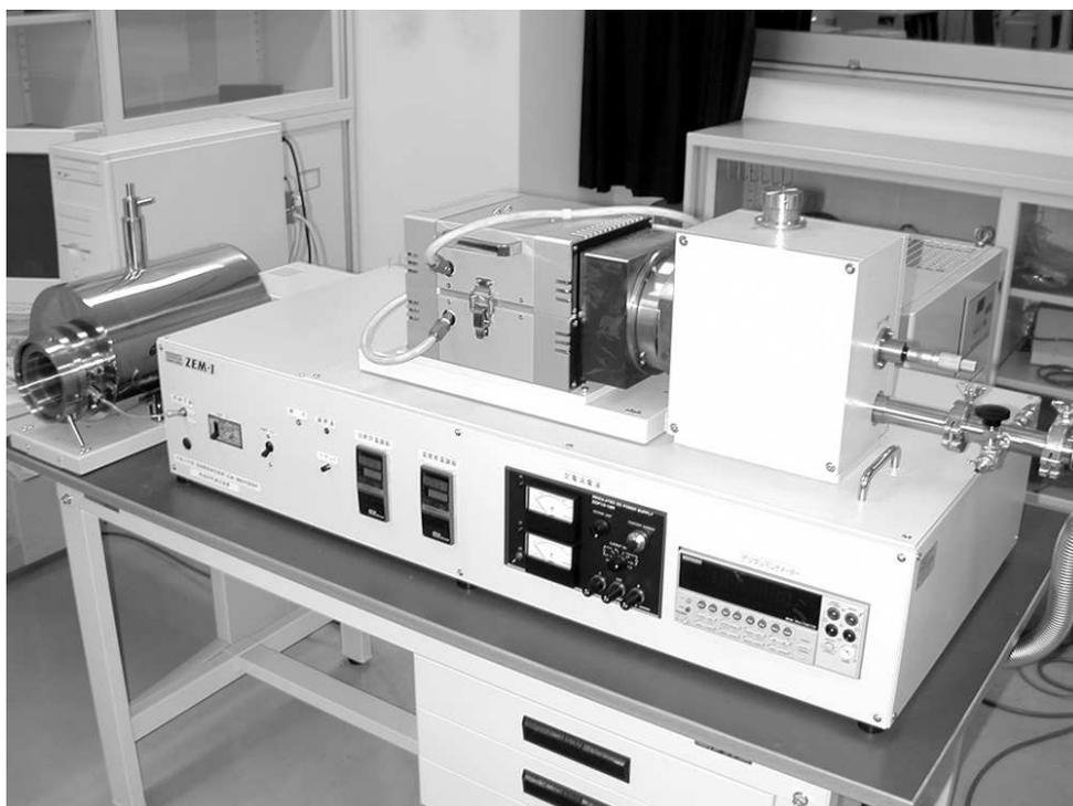
Fig. 3.1. Appearance of thermoelectric measurement apparatus.
