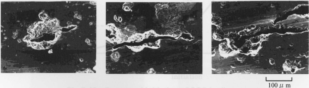
Fig.7-10 Microcracks from corrosion pit after cleaning
