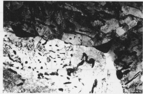
Grain boundary carbides are large
