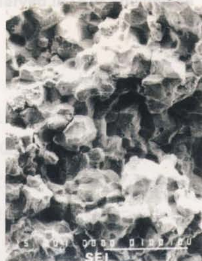
Fig.3-6 DUB specimen fracture surface showing initiation from corrosion pit and intergranular fractures
