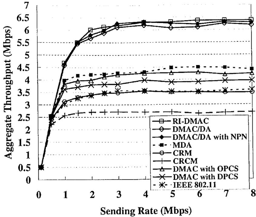
Figure 5.34: Throughput in scenario where flows are randomly changed.
