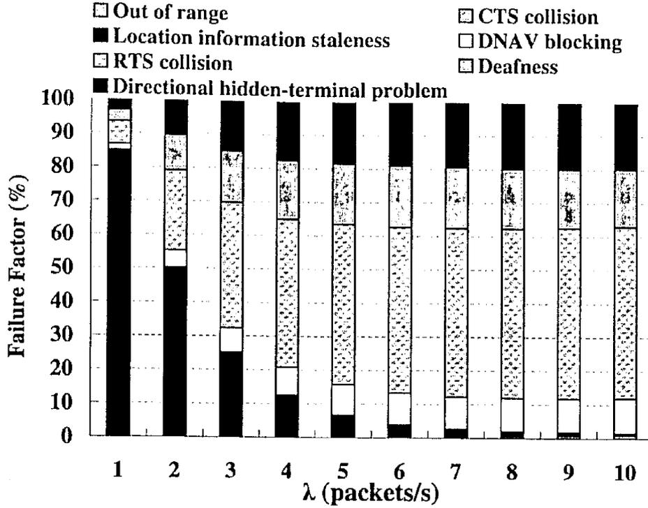
Figure 4.24: Communication failure factors of SWAMP (OC+EC).
