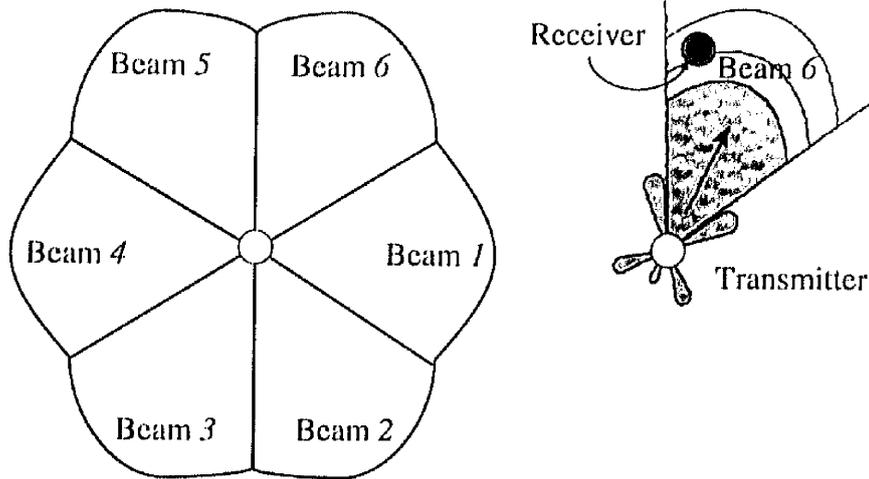
Figure 3.2: Switched beam antenna with 6 beams.
