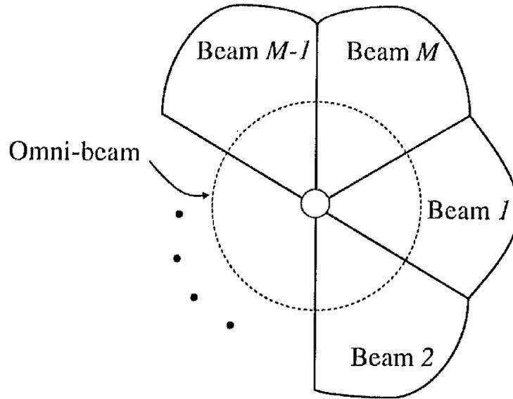
Figure 5.4: Antenna model with M beams.
