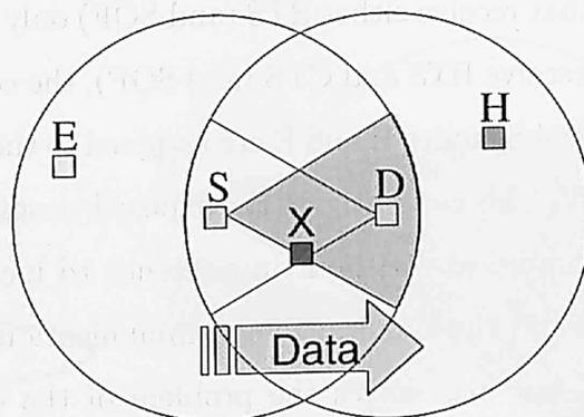
Node S transmits Data using directional beam DL towards D
