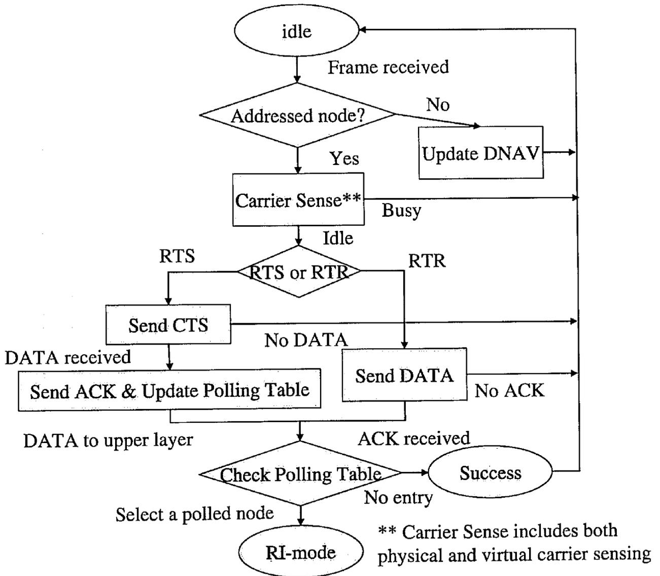
Figure 5.11: Flowchart of RI-DMAC (Receiver side).
