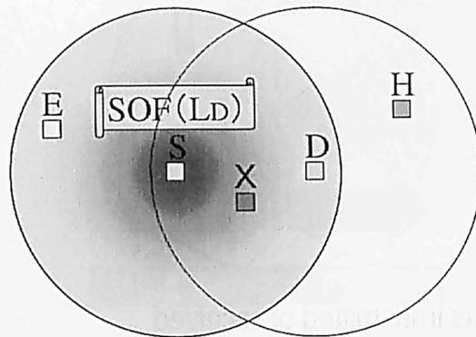
Node S transmits SOF (Start of Frame) with  $L_D$  using omni-directional beam
