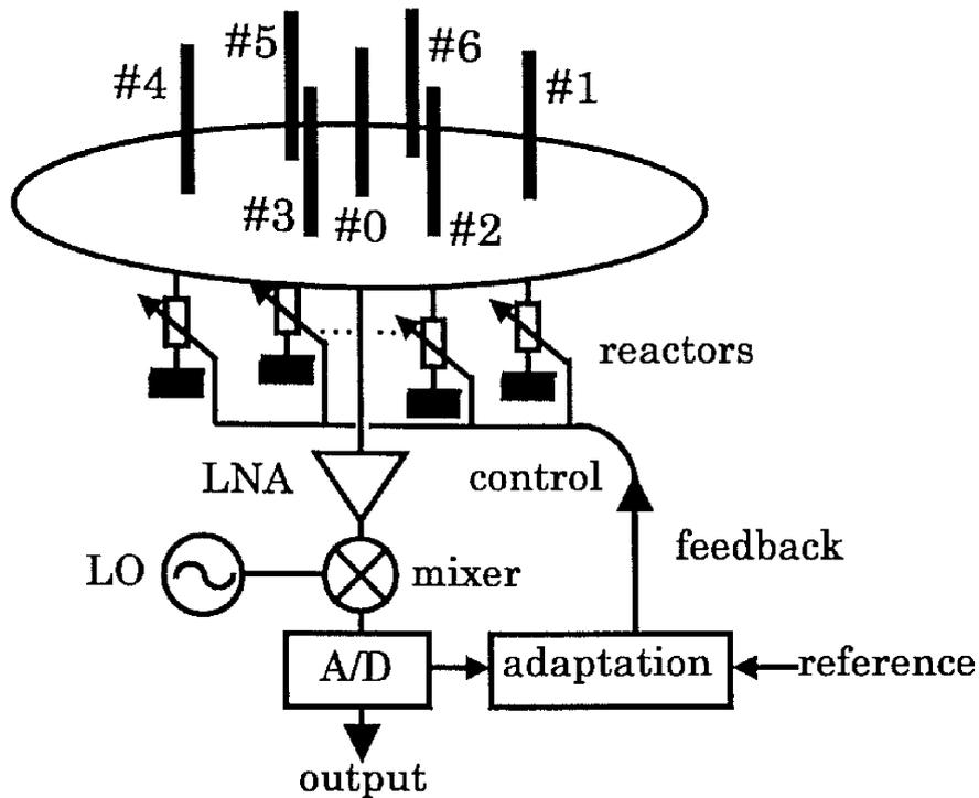
Figure 3.5: Configuration of ESPAR antenna.
