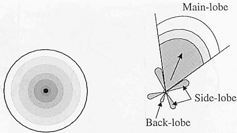
A. Omni-directional antenna      B. Directional antenna
