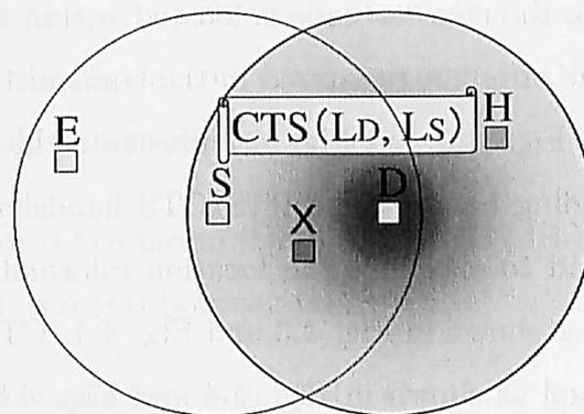
Node D transmits CTS with  $L_D$  and  $L_s$  using omni-directional beam
