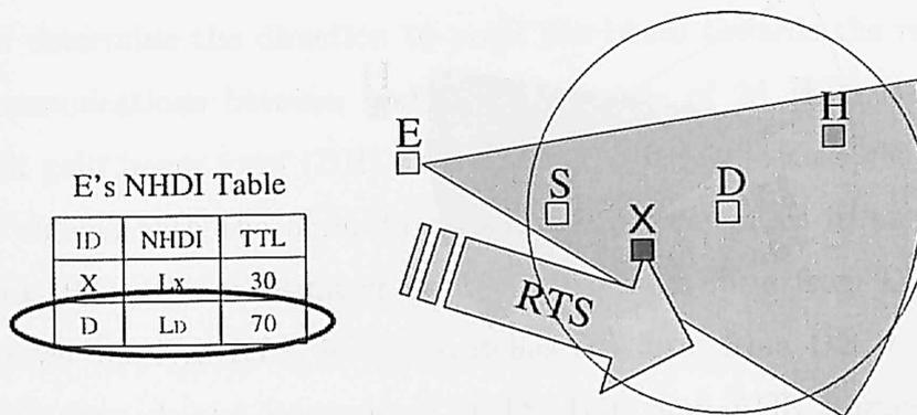
Node E transmits RTS using directional beam DH towards D based on own NHDI table information
