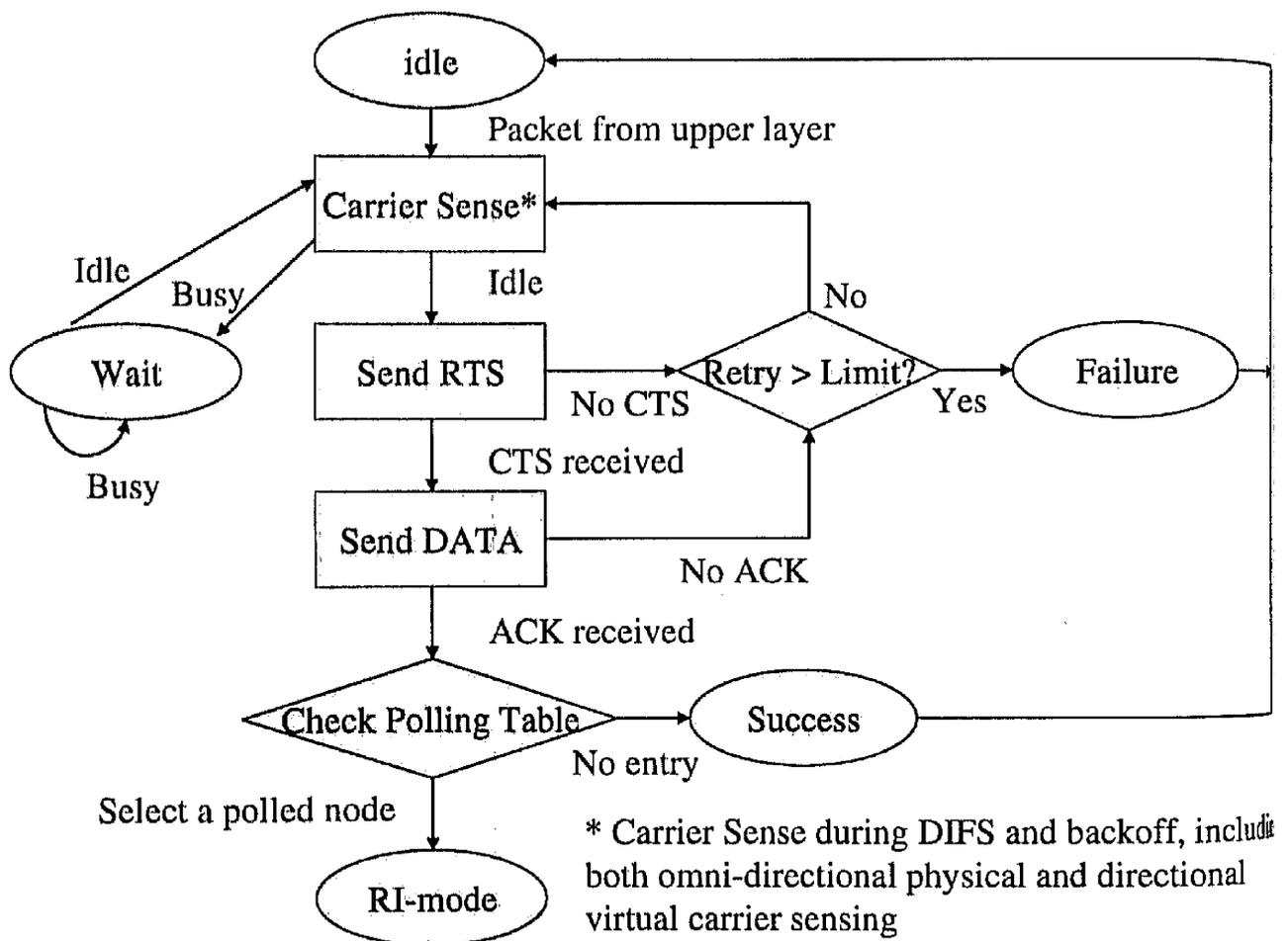
Figure 5.10: Flowchart of RI-DMAC (Sender side).
