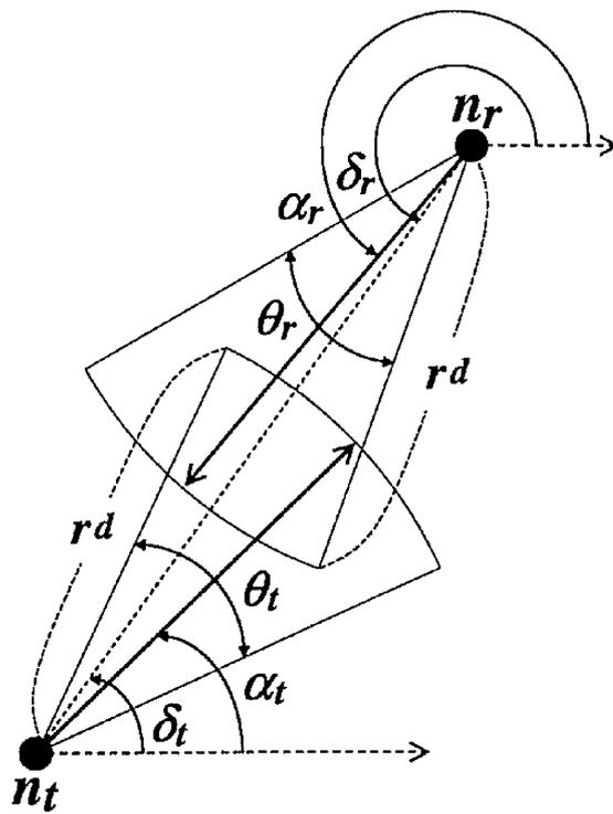
Figure 3.9: Definition of directional communication.
