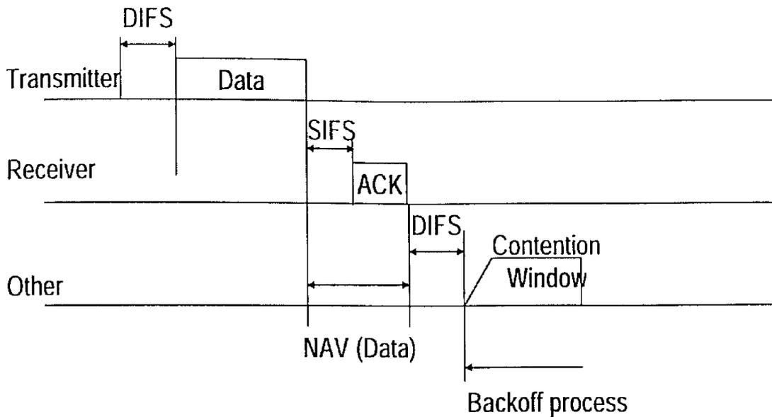
Figure 2.7: Basic access method in DCF.
