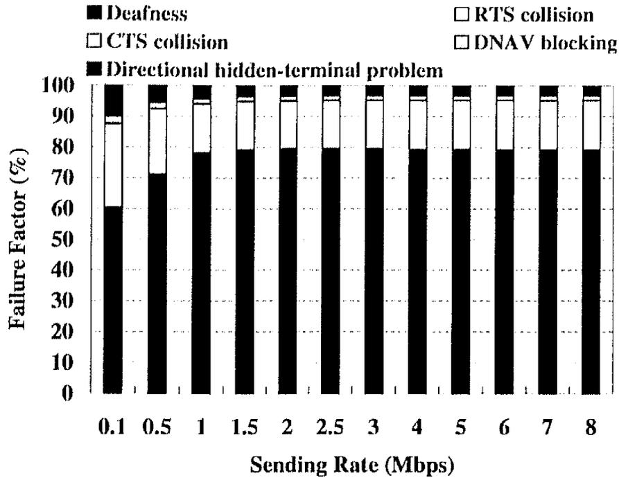
Figure 5.1: Communication failure factors of DMAC.
