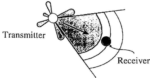
Figure 3.3: Steered beam antenna.
