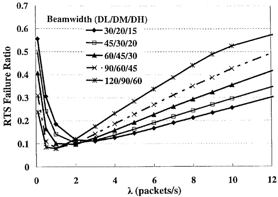
Figure 4.26: Effects of the beamwidth on RTS failure ratio.
