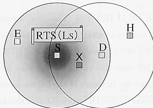
Node S transmits RTS with  $L_s$  using omni-directional beam
