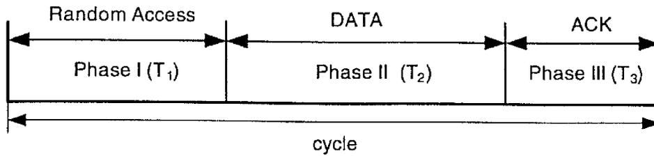
Figure 3.20: Timing structure of SYN-DMAC.
