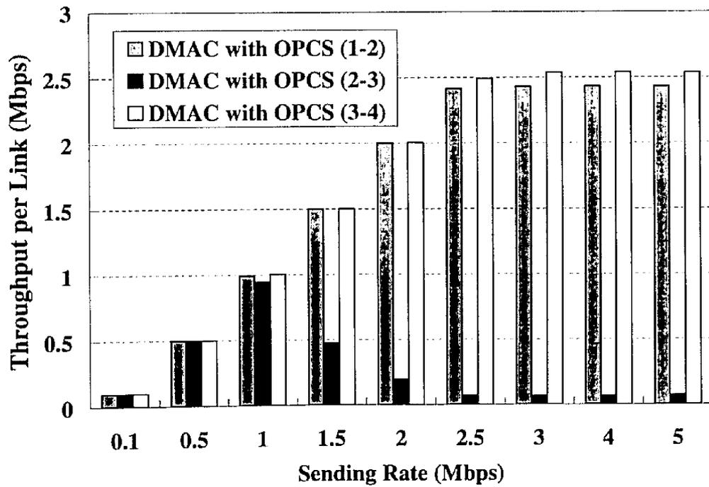
Figure 5.19: Link throughput of DMAC with OPCS.
