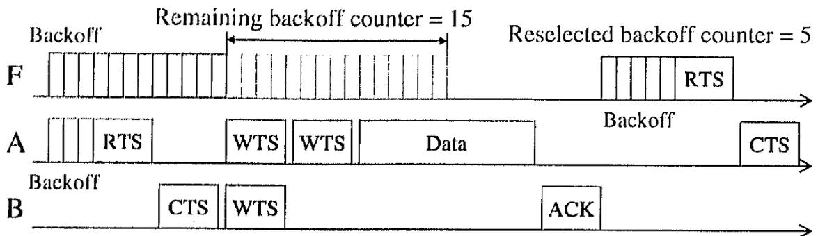
Figure 5.6: Handling the wastage of the wireless channel.
