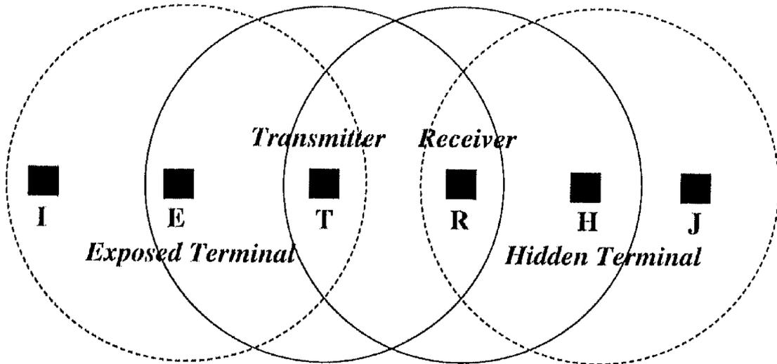
Figure 2.4: Hidden-terminal and exposed-terminal problems.
