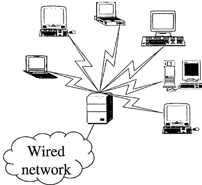
Figure 2.2: Centralized wireless networks.
