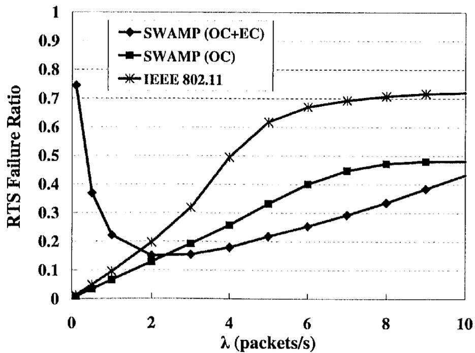
Figure 4.23: RTS failure ratio.
