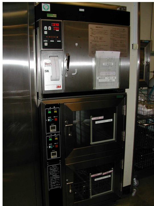
Fig. 1.2 Photograph of a commercial EOG sterilizer (3M) used in the hospital (by courtesy of Hamamatsu University School of Medicine).
