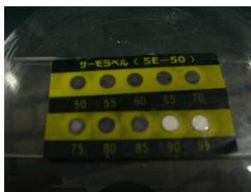
Fig. 5.2 Thermo-label sheets, 5E-50 and 5E-75.
