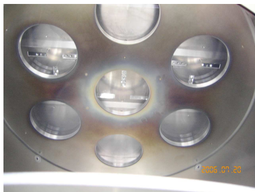
Fig. 3.5 Photograph of the seven small quartz windows.
