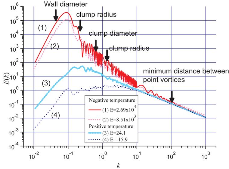
Figure 11: Energy spectra are plotted at various temperatures. The temperature is controlled by the initial configuration of the vortices.
