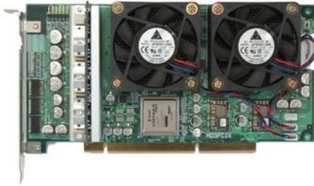
Figure 4: MDGRAPE-3 is a PCI-X card.
