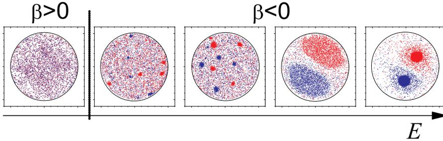
Figure 8: Equilibrium distributions of the vortices are shown. In the right edge distribution, the upper and lower clump exclusively consists of the positive and negative vortices, respectively.
