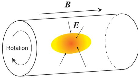
Figure 1: Schematic of confinement geometry is shown. Strong axial magnetic field and edge electrostatic potential confines electrons. They rotate in  $\mathbf{E} \times \mathbf{B}$  direction.
