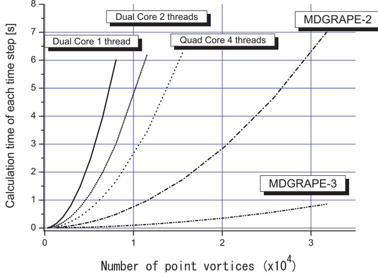
Figure 5: Calculation time per one time step is plotted against the number of point vortices without image vortices.
