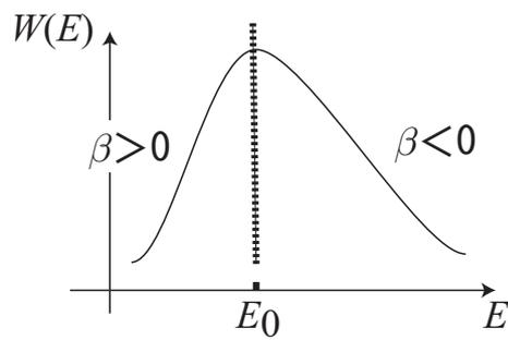
Figure 3: The density of state has at least a peak when the total number of states is limited. In this case, negative temperature state appears when  $E > E_0$ .
