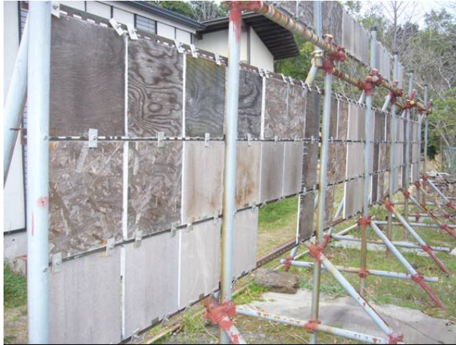
Fig. 1. Outdoor exposure test conducted in Shizuoka.
