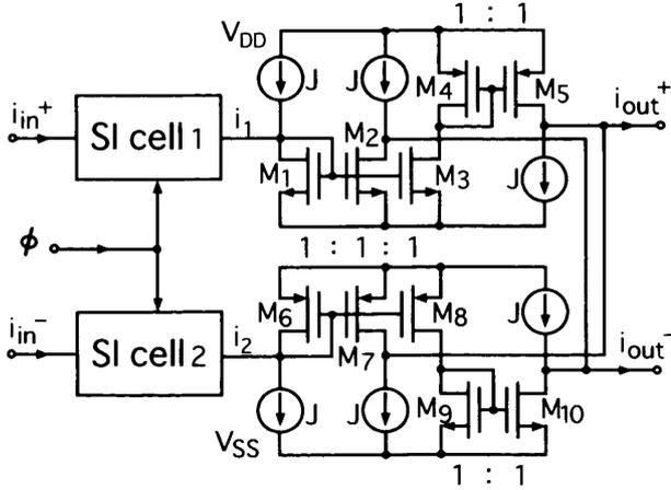
Fig. 2 Proposed fully-differential SI circuit.
