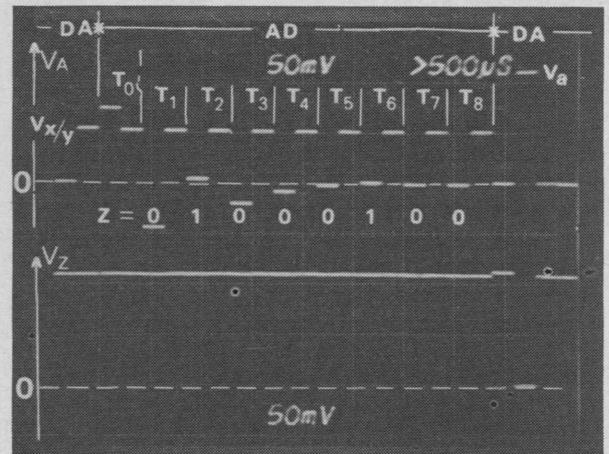
Fig. 8. Waveforms appearing when the digital operation  $(1000) \div (1111)$  was executed. Upper trace: The voltage at node (A) during the XEC state. Lower trace: The output voltage of S/H circuit. (The actual vertical scale is ten times that indicated in the figure, since a 10:1 oscilloscope probe was used.)
