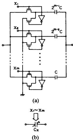
Fig. 1. An  $m$ -bit programmable binary-weighted capacitor array (a) and its symbol (b).
