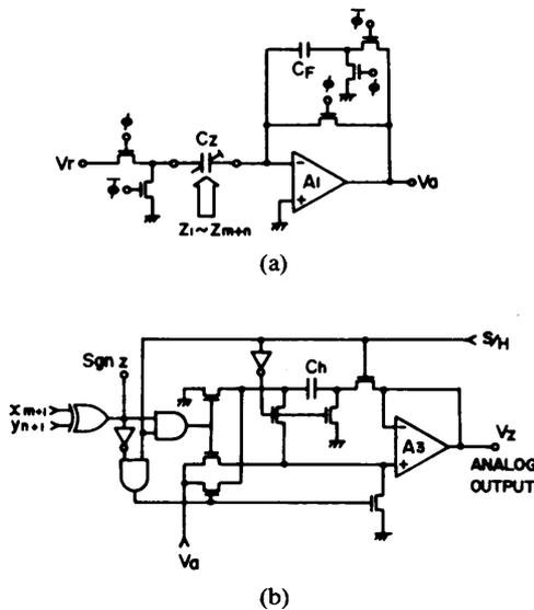
Fig. 5. Circuit configurations for analog output: (a) The D/A converter in the  $T_{m+n+1}$  period. (b) The sample and hold circuit.
