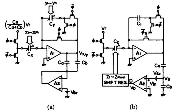
Fig. 4. Circuit configurations for division: (a) The D/A converter (DA state). (b) The successive-approximation A/D converter (AD state).
