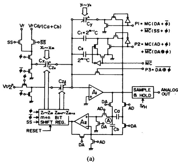
Fig. 2. (a) The schematic diagram of the switched-capacitor digital multiplier/divider, where AD, DA, and SS are the state signals controlling its operation. Their timing sequence is shown in (b).
