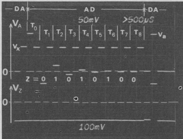
Fig. 7. Waveforms appearing when the digital operation  $(-0111) \times (1100)$  was executed. Upper trace: The voltage at node (A) during the XEC state. Lower trace: The output voltage of S/H circuit. (The actual vertical scale is ten times that indicated in the figure, since a 10:1 oscilloscope probe was used.)
