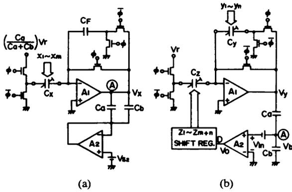
Fig. 3. Circuit configurations for multiplication: (a) The D/A converter (DA state). (b) The successive-approximation A/D converter (AD state).
