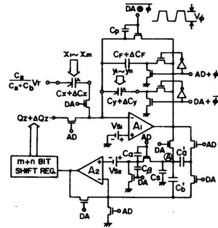
Fig. 6. The schematic diagram of the multiplier circuit including the important parasitic elements.
