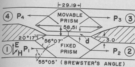
Fig. 1. Sectional view of the directional coupler.
