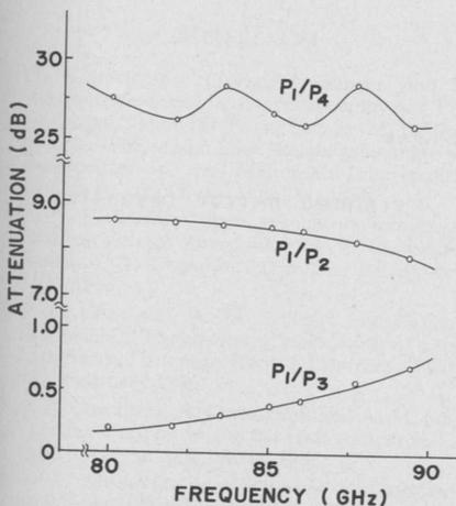
Fig. 4. Frequency characteristics of the directional coupler;  $d/\lambda = 0.03$ .
