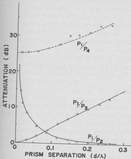
Fig. 3. Transmission characteristics of the directional coupler as a function of  $d/\lambda$ . Solid lines: theoretical values. Circles: experimental values obtained at 87 GHz.
