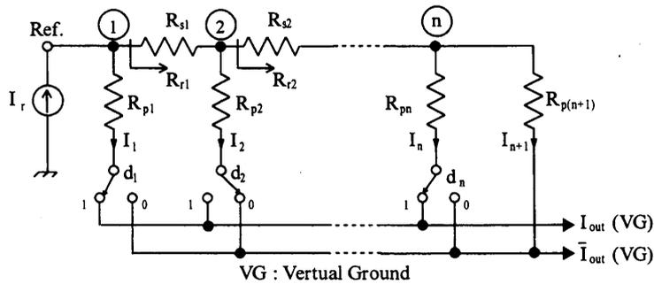
Fig. 3. Current-mode R-2R ladder D/A converter.
