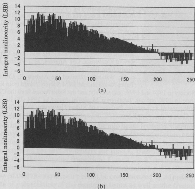
Fig. 11. Integral nonlinearity of the prototype D/A converter: (a)  $I_r = 256 \mu\text{A}$ ; (b)  $I_r = -256 \mu\text{A}$ .  $W/L = 200 \mu\text{m}/3 \mu\text{m}$ .
