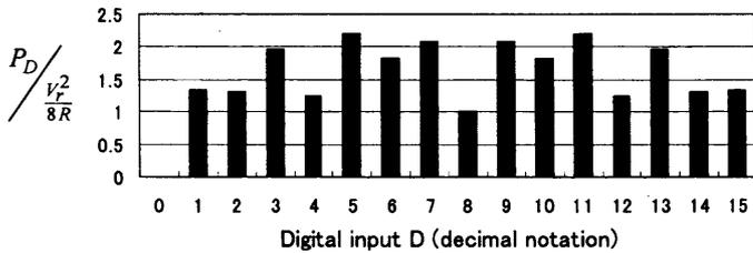
Fig. 2. Normalized power dissipation of a 4-bit R-2R ladder D/A converter as a function of the digital input.
