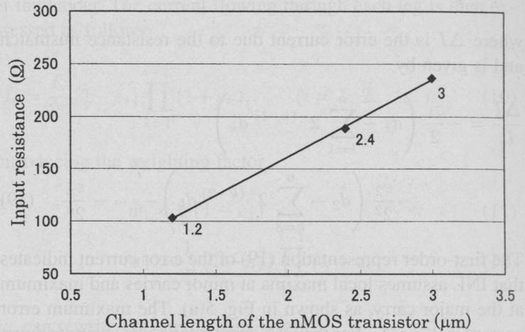
Fig. 9. The equivalent resistance versus the gate length of an nMOS transistor.
