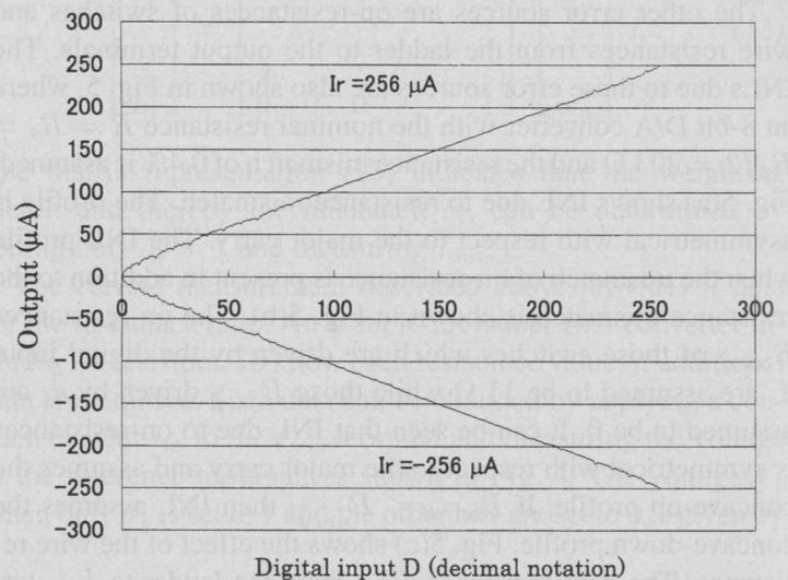
Fig. 10. Transfer characteristics of the prototype D/A converter:  $W/L = 200 \mu\text{m}/3 \mu\text{m}$ .
