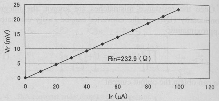
Fig. 8. Current versus voltage characteristics at the reference node.
