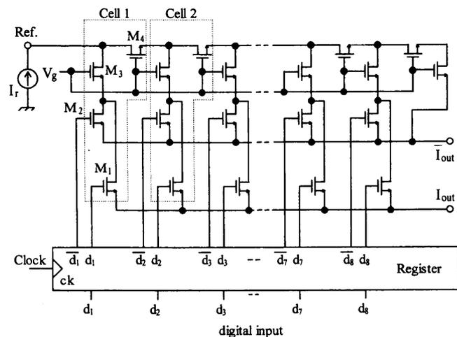
Fig. 6. Circuit diagram of an 8-bit D/A converter fabricated by  $0.6 \mu\text{m}$  CMOS process.
