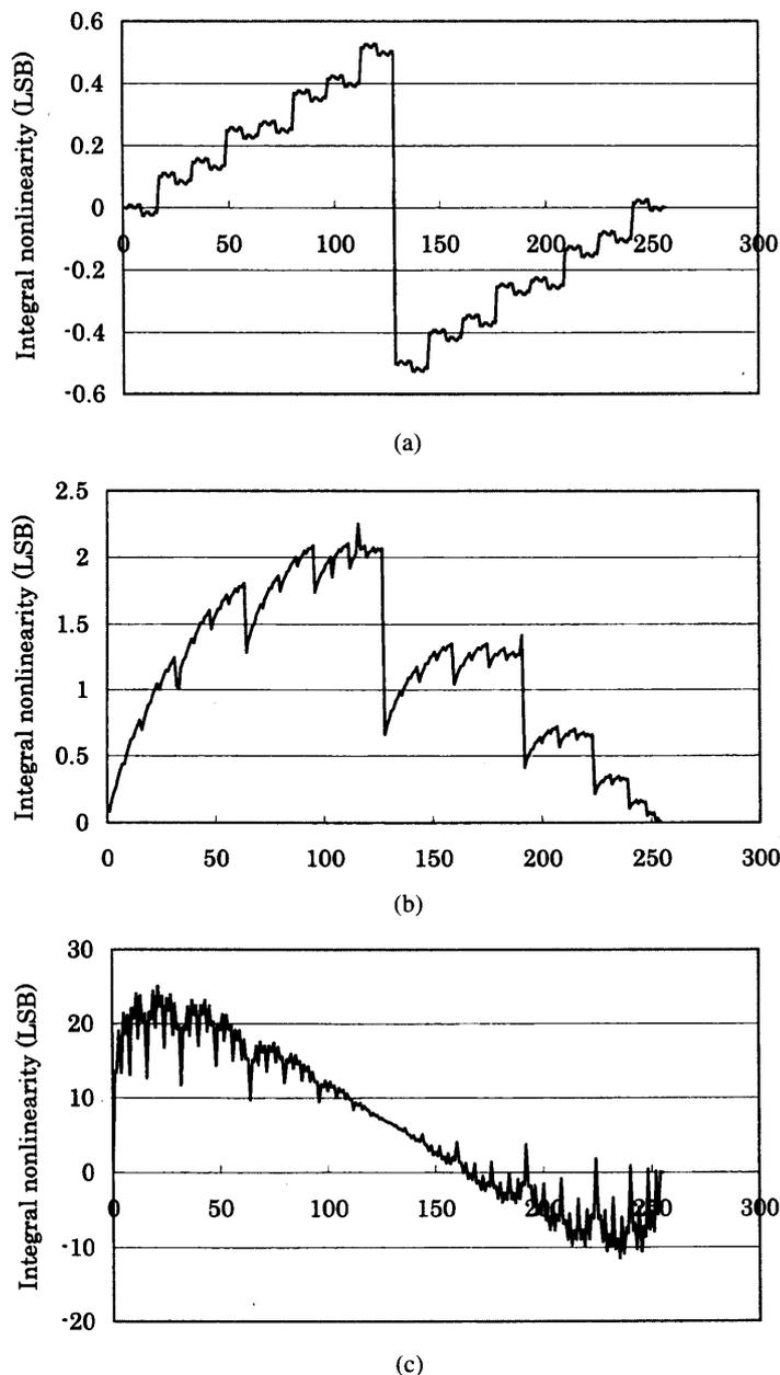
Fig. 5. INL profiles due to mismatches in (a) resistance, (b) on-resistance of switch, and (c) wire resistance.
