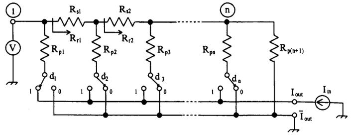
Fig. 4. D/A converter under resistance measurement.
