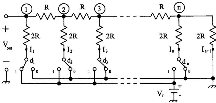
Fig. 1. Voltage-mode R-2R ladder D/A converter.
