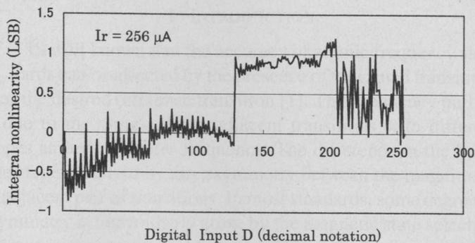
Fig. 12. Integral nonlinearity of the CMOS ladder.  $W/L = 200 \mu\text{m}/3 \mu\text{m}$ .
